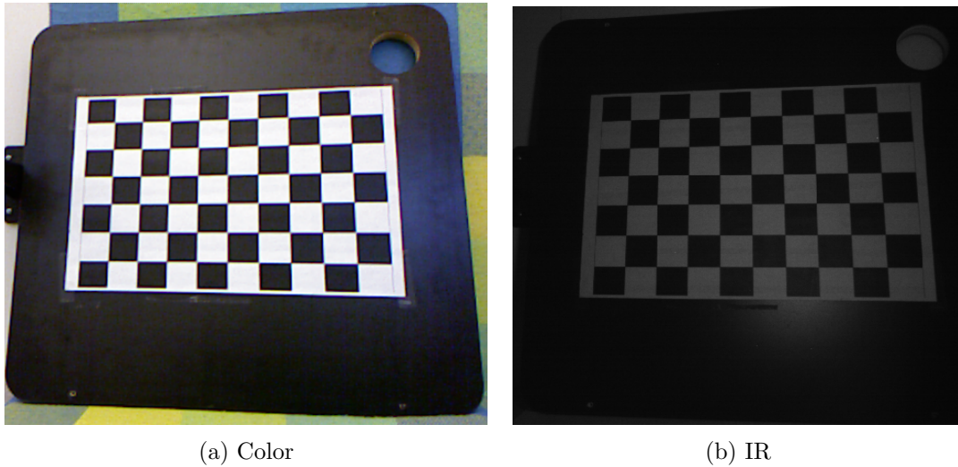
Figure 4.9: Checkerboard pattern used to calibrate the Kinect.
