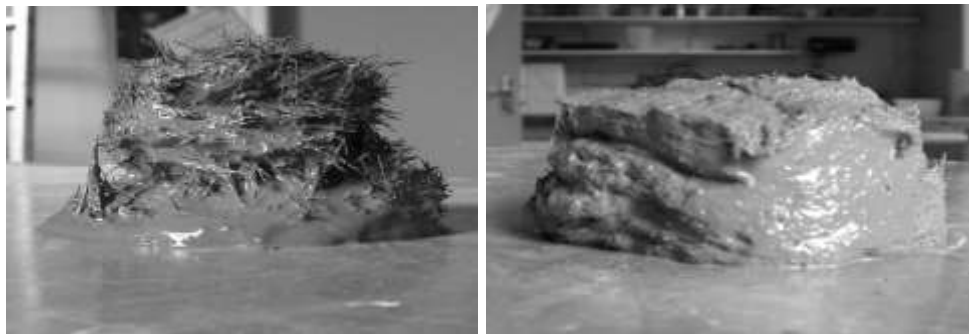
Figure 2.14 Consistency of cement paste mixed with fibers having various aspect ratios and water-cement ratio of 0.4 (Martinie et al. 2009)
