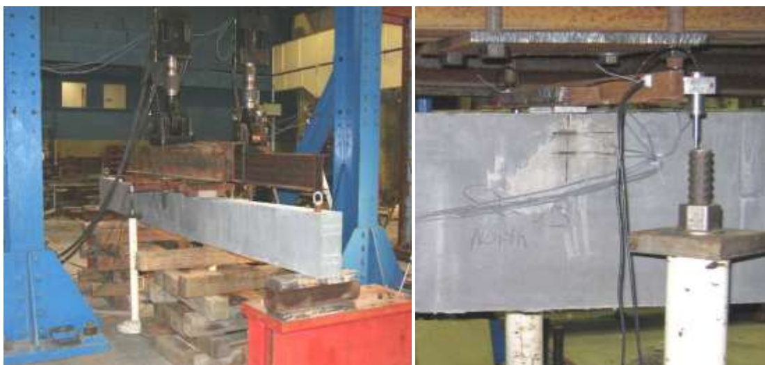
Figure 2.22 The flexural test set-up (Meade and Graybeal 2010)
