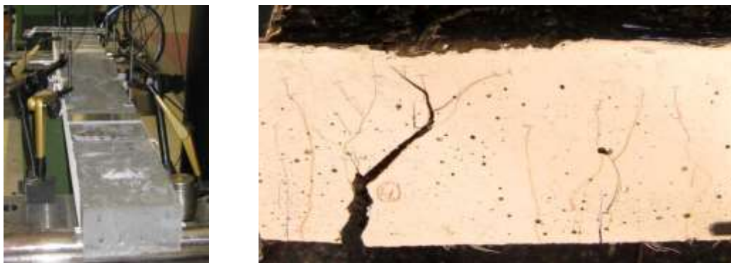
Figure 2.20 Four-point-bending test; test setup and crack pattern (Fehling et al. 2010)
