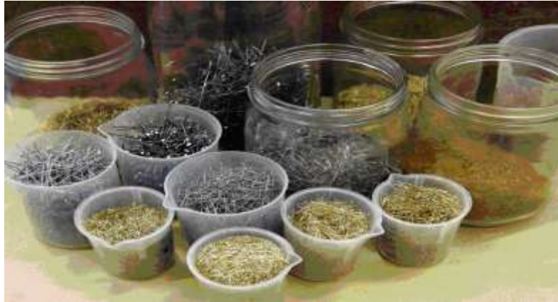
Figure 2.12 Different fiber types used for fiber reinforced concrete (Martine et al. 2009)
