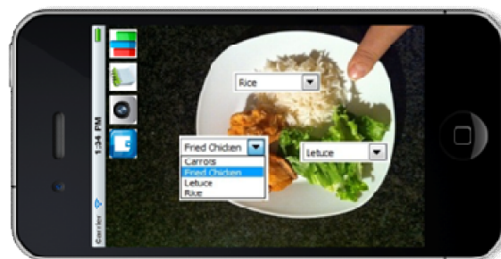
Figure 6-5 The SVM module verifies with the user the type of foods it has determined.
