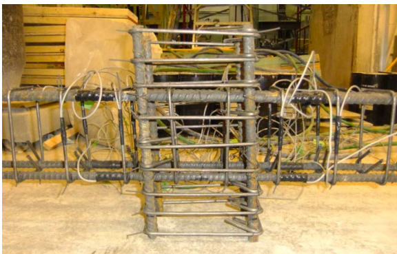
Figure 3.7 Typical cage showing strain gauge instrumentation
