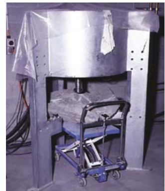
c) Round panel test rig with tested specimen
