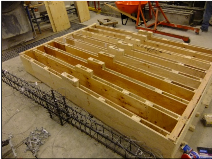
Figure 3.10 Formwork used to cast concrete beam specimens
