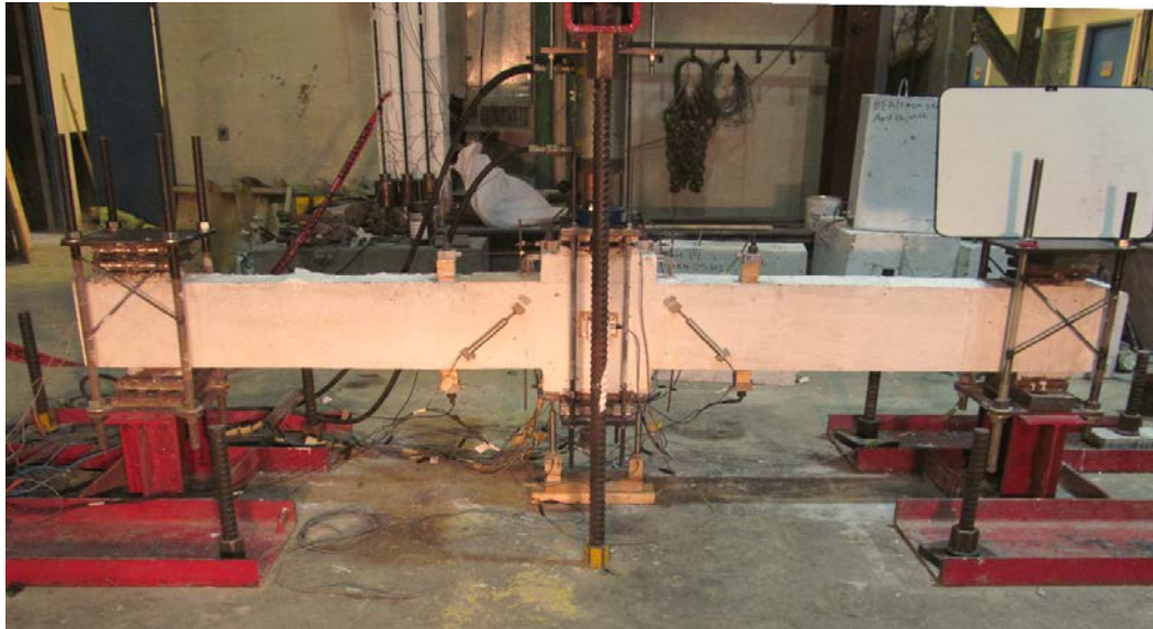
Figure 3.16 Beam specimen prior to testing
