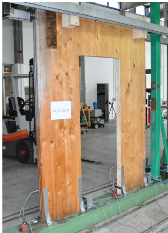
Figure C-2. Measuring device disposition of shearwall 1. Sketch (a) and photo (b)
