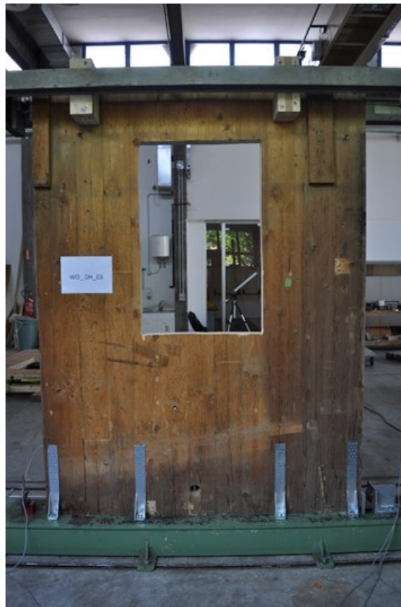
Figure C-10. Measuring device disposition of shearwall 3. Sketch (a) and photo (b)
