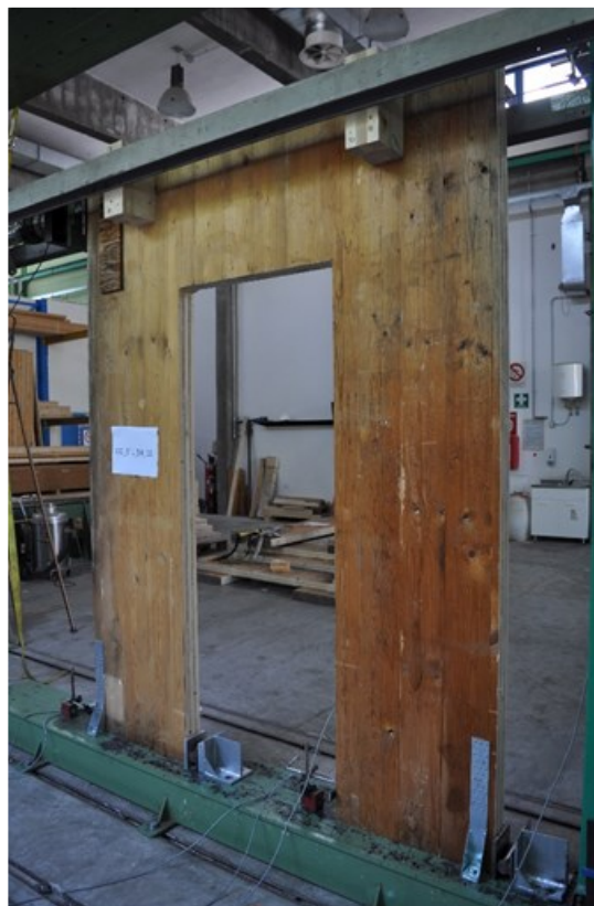
Figure C-6. Measuring device disposition of shearwall 2. Sketch (a) and photo (b)
