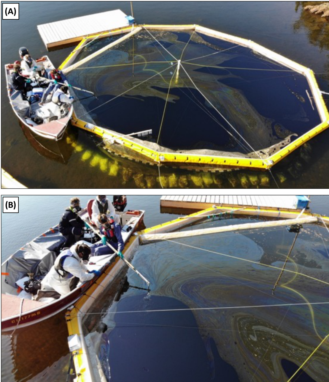
Figure S1. The addition of 180 L of CLWB (1:590 oil:water, v/v) onto the water surface of the limnocorral. (A) Overview of addition method, (B) View of telescopic arm and pumping system being held at approximately 5 – 10 cm from the water's surface. The oil exited the hose parallel to the water's surface to avoid forcing oil below the water surface and allowing it to spread out during the addition.
