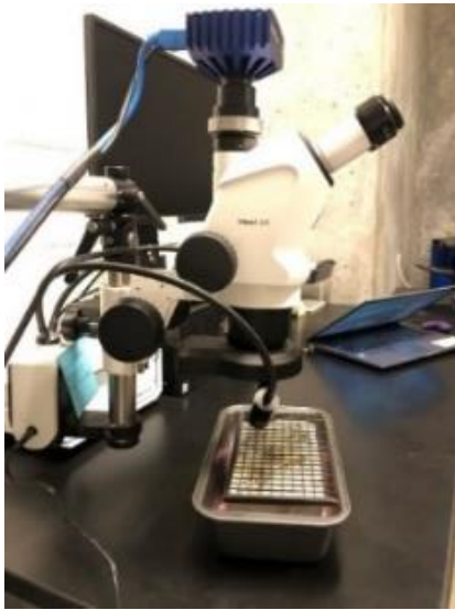
Figure 5.2. a) Stereomicroscope and specimen/core set-up and b) illustration of crack counting method on 1 cm 2 micrograph taken from a core under analysis in this current work. The black solid line represents a grid line to demonstrate the crack counting method considering adjacent squares for the particle's Debon-type crack.
