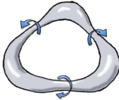
Figure 6.16: Sketch of inferred vortex ring shape without the effects of valve orientation.
