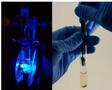
Figure 5.1. Picture showing the reaction setup used under LED irradiation and continuous stirring (left), and the easy removal of the GW material from the reaction vessel utilizing a pair of tweezers (right).
