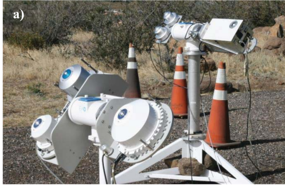
Fig 1. a) Two SolarSIM-Gs were calibrated against the EKO WISER and LICOR Li-1800 spectroradiometers in the global normal orientation at the Solar Radiation Research Laboratory (SRRL). b) Two SolarSIM-Gs were deployed in the global horizontal orientation post-calibration at the SRRL to assess their broadband and spectral performance against NREL's pyranometers and spectroradiometers, respectively.
