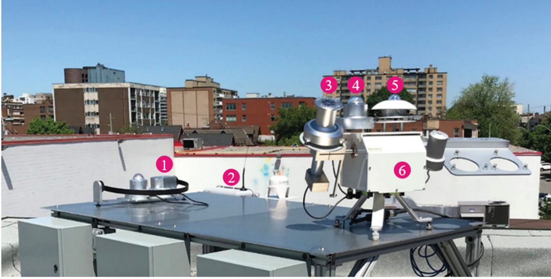
FIGURE 1. Solar test site in Ottawa consisting of Spectrafy's spectral instruments: the SolarSIM-D2 (3), the SolarSIM-G (4), and the SolarSIM-E (1), Huksenflux's SR20 pyranometer (5), Geonica's datalogger (2) and SEMS-2000 solar tracker (6).
