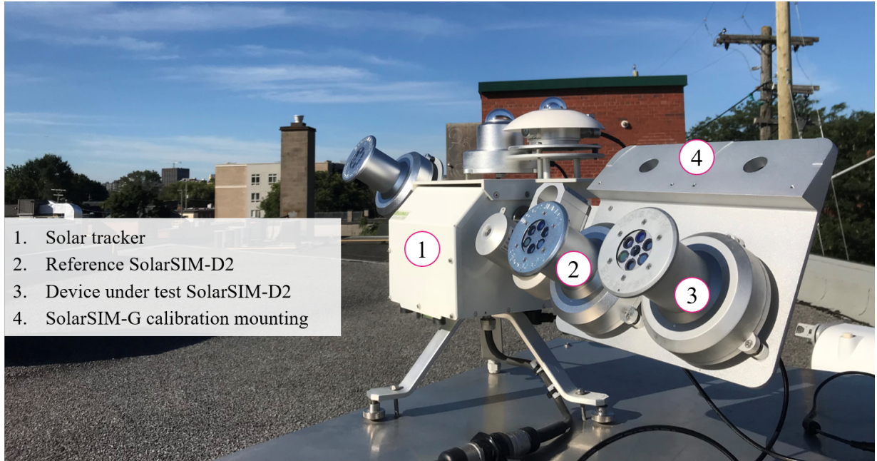
Figure 3.3: Optical calibration setup for either the SolarSIM-D2 (as shown) or the SolarSIM-G.
