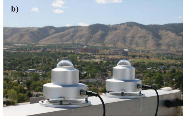
Fig 1. a) Two SolarSIM-Gs were calibrated against the EKO WISER and LICOR Li-1800 spectroradiometers in the global normal orientation at the Solar Radiation Research Laboratory (SRRL). b) Two SolarSIM-Gs were deployed in the global horizontal orientation post-calibration at the SRRL to assess their broadband and spectral performance against NREL's pyranometers and spectroradiometers, respectively.
