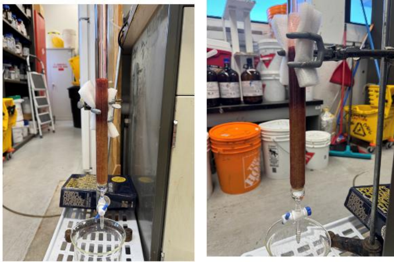
Figure 12.15. Column study at a flow rate of 1 mL/min with a pH of 4 and a dilution factor of 4.
