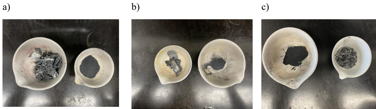
Figure 12.3. Heat-treated cathode materials (separated black mass and Al) a) 600°C in the air atmosphere in 6h b) 650°C in the air atmosphere in 6h, and c) 600 °C in the air atmosphere in 4h.
