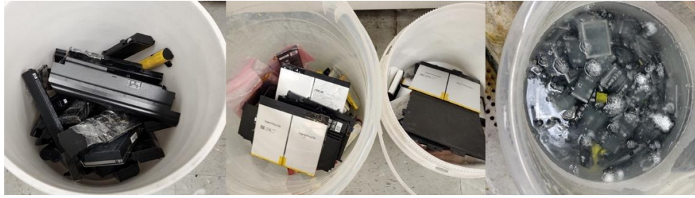
Figure 3.2. The collected Li-ion batteries (Left-hand side: laptop batteries, middle: Li-polymer batteries, right-hand side: cellphone batteries).
