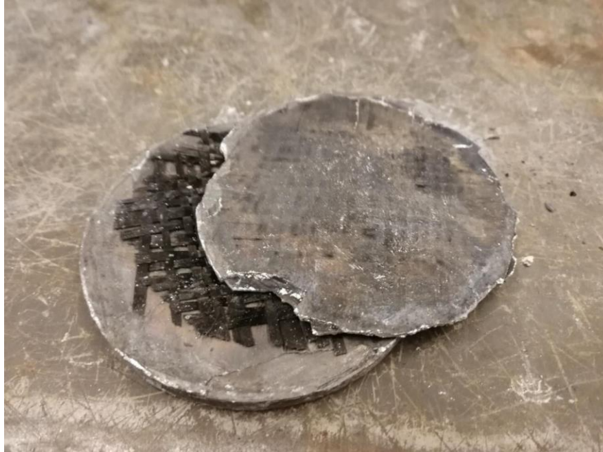
Figure 4-2: Brittleness and lack of aluminum-fiber bonding in samples fabricated using Copper and Brass foils as seal.
