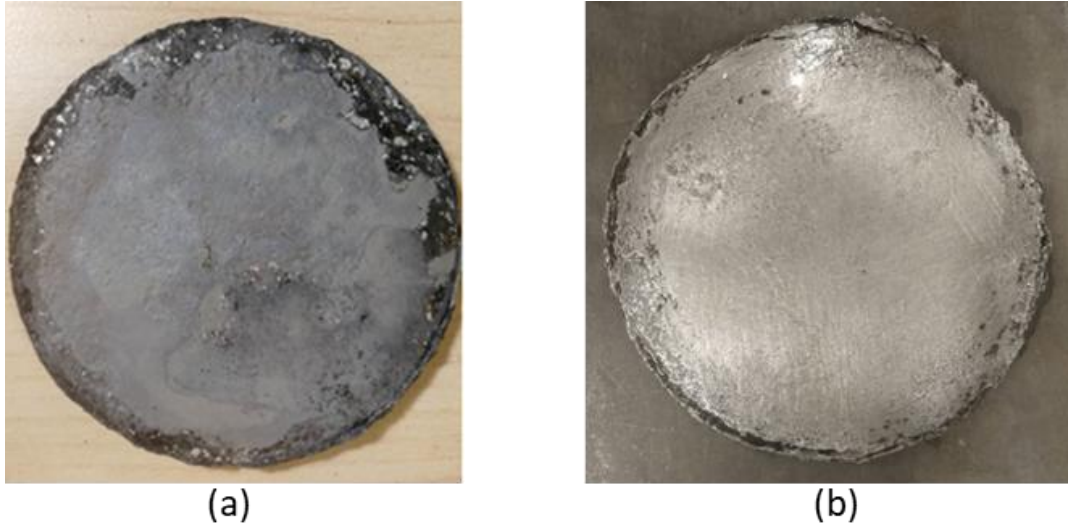
Figure 4-1: (a) As-cast composite sample and (b) after surface cleaning
