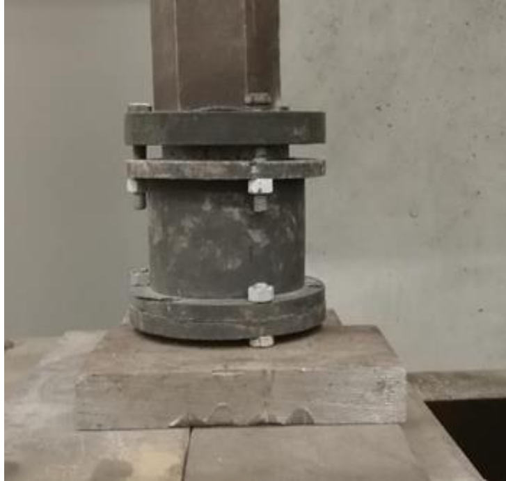
Figure 3-9: Pressure application on the die set-up using a hydraulic press during cooling
