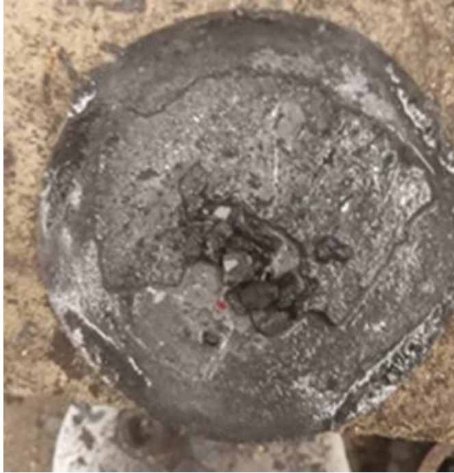
Figure 4-3: High hydraulic pressure of 90 MPa caused the decomposition of carbon fiber and their reaction into graphite or carbide particles.
