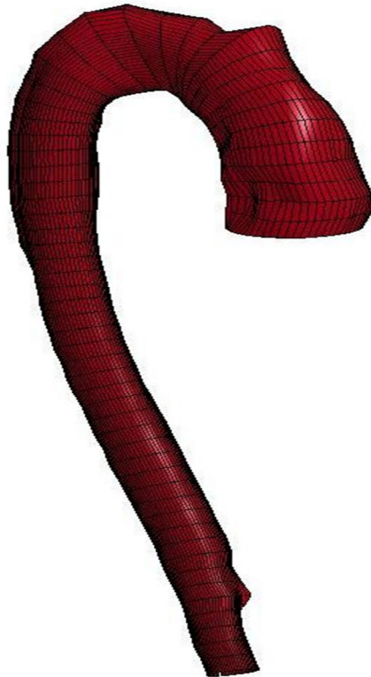
Figure 5.36: LS-DYNA mesh for descending thoracic aortic aneurysm dataset.
