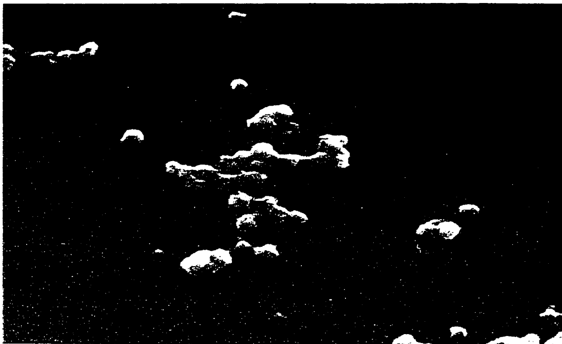
Figure 4.14 SEM image of the internal surface of a modified cellulose acetate (MCA) dialysis hollow fiber membrane.
