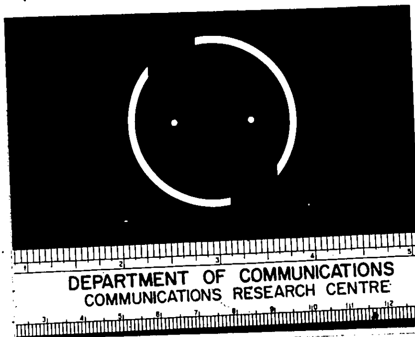
Fig. 5-3 A view of the ground plane of circuit MIC-034 showing the coupling apertures and mode suppressor.
