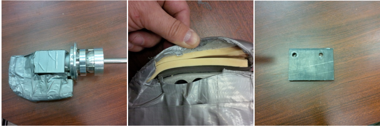
Figure S1-4. Impacting anvil used to simulate a punch. Foam layers can be seen in second photo. The final photo shows a 500 gram mass that can be added to the anvil to adjust the impact mass.
