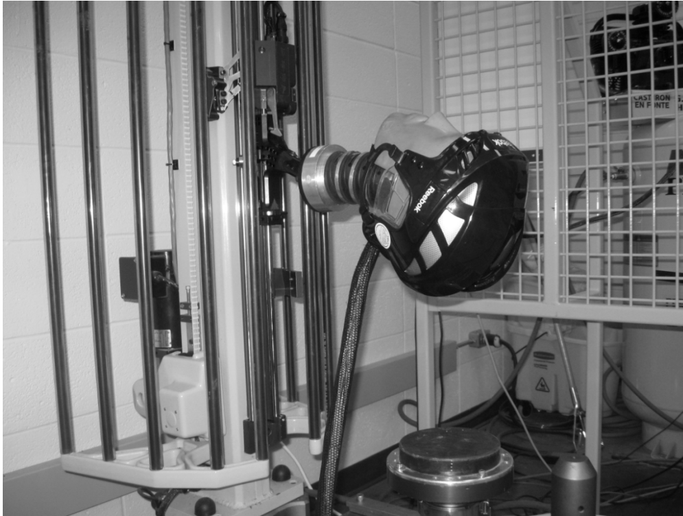
Figure S1-1. Example of a monorail drop system used to simulate a head impact to the ice.
