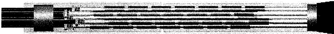
Figure 5.8: Schematic of revised multi-strand steel meso-rod specimen with glass mould and predefined break at the centre. An exploded view detailing the sealing mechanism is shown in Figure 5.9
