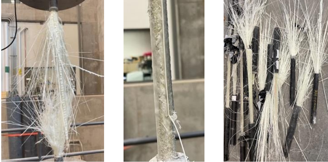
Figure 4-1. Overview of sample failures, and fibre cable breakage
