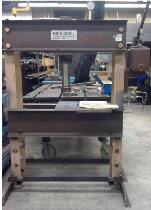
Figure 3-8: Hydraulic press (50 ton) for squeeze casting setup.
