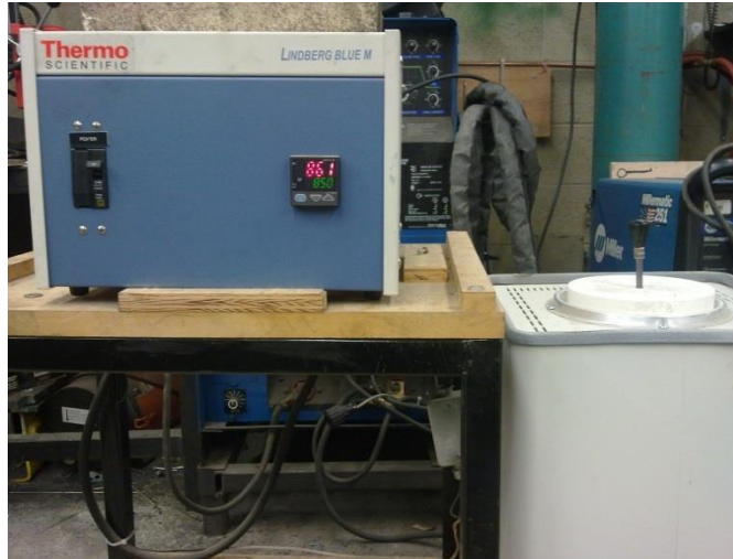
Figure 3-4: Lindberg vertical furnace used to melt aluminium 6061.
