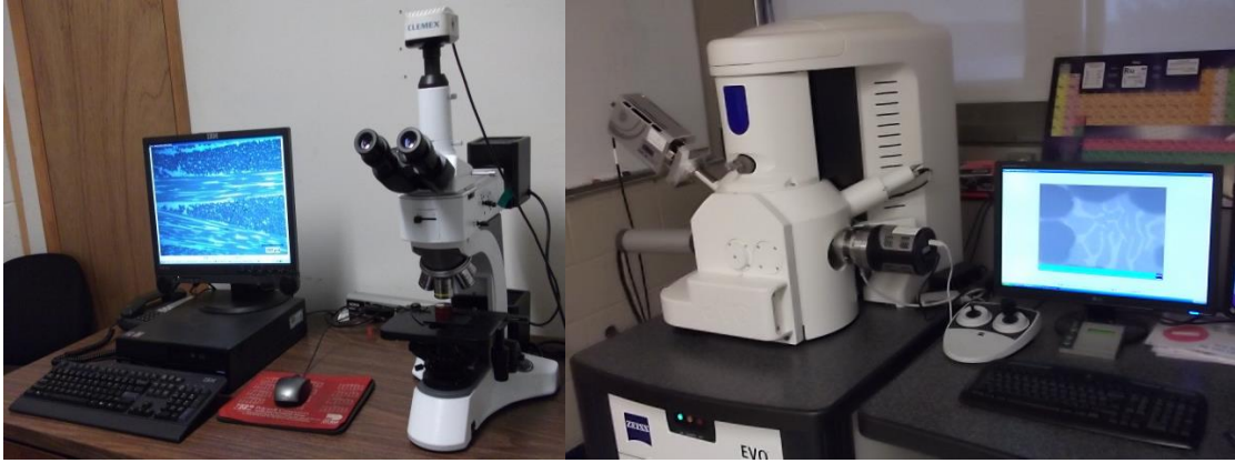
Figure 3-18: XJP-3A optical microscope (left) and ZEISS electron microscope (right) used for microscopy.
