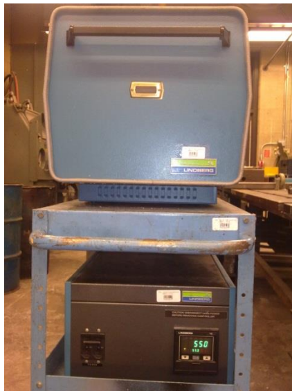
Figure 3-5: Lindberg horizontal furnace used to preheat the fiber preform.
