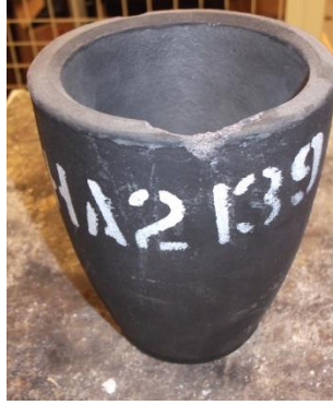
Figure 3-6: Graphite crucible cup to handle the molten aluminium alloy.
