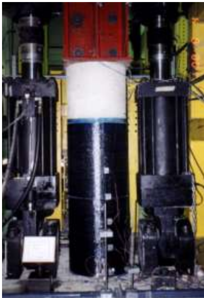
c) Retrofitted column BR-C8-1 (4 plies of CFRP)
