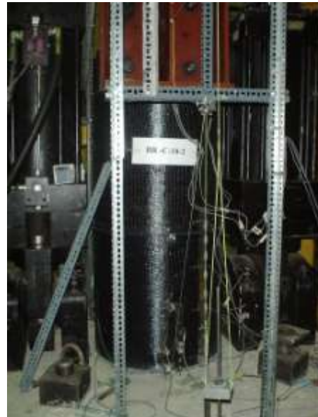
Retrofitted column BR-C10-2 (2 plies of CFRP)
