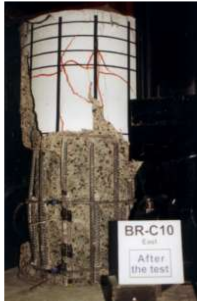
Control column BR-C10 after test
