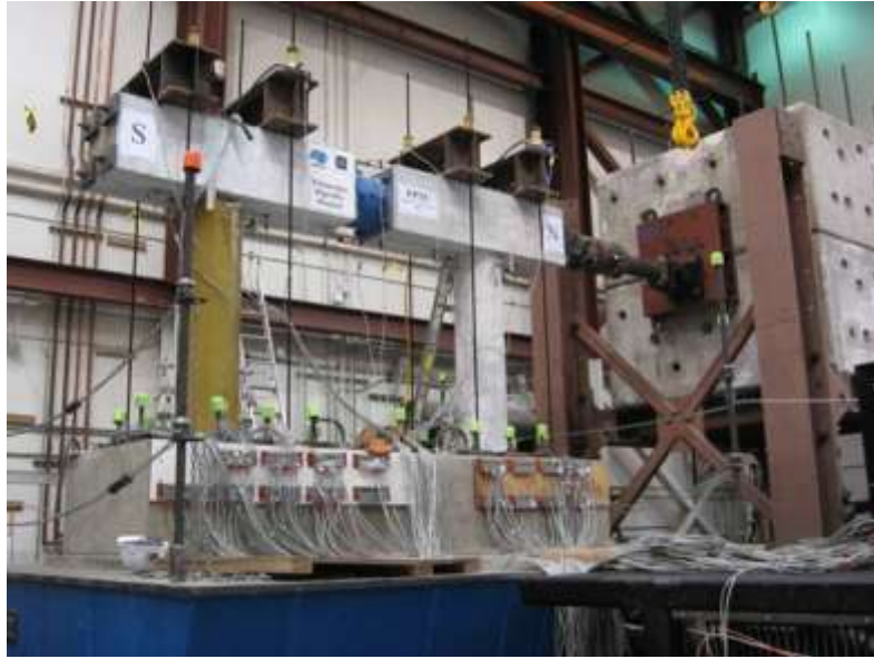
Fig. 1.17 Two-column piers shake table setup
