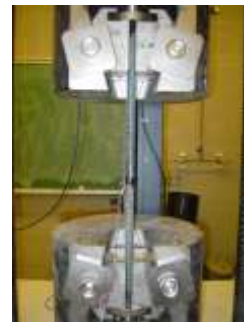
Sample ready for tension test
