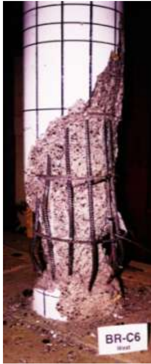
Control column BR-C6 after test
