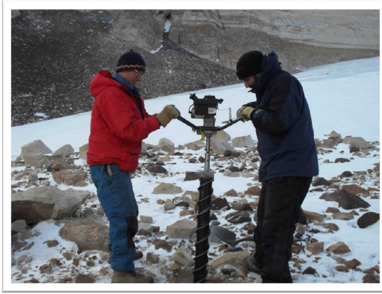
Figure 9: Photo illustrating field sampling of permafrost cores using the CRREL drill in University Valley, McMurdo Dry Valleys of Antarctica (Photo Source: Dr. Denis Lacelle).
