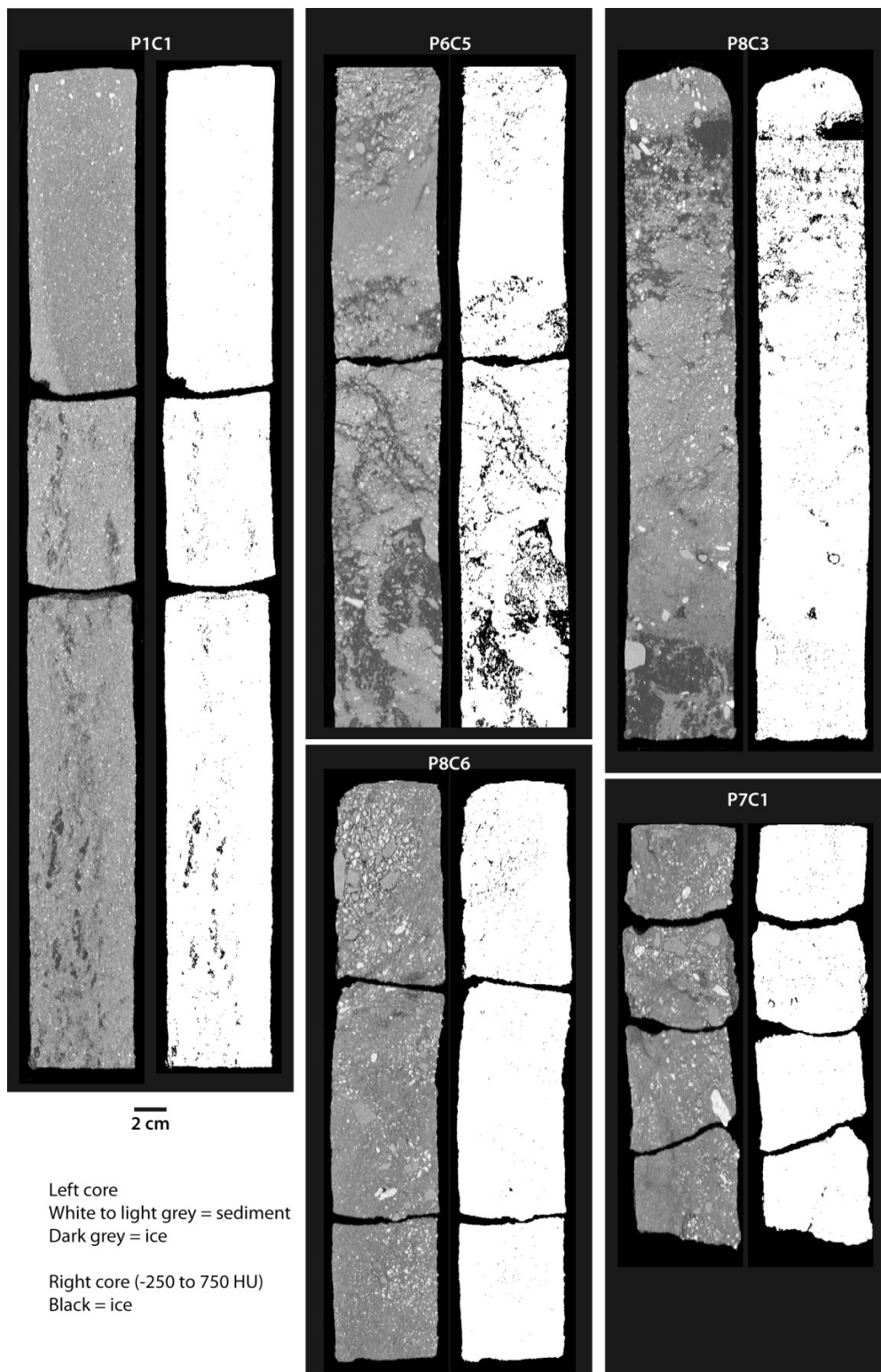
Figure 29: Montage of sample binary image slices for cores P1-C1, P6-C5, P8-C3, P8-C6 and P7-C1 illustrating crustal, suspended and structureless cryostructures.
