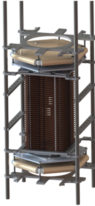
FIGURE 3.9: The design schematic of the COLTRIMS spectrometer. A constant voltage is applied across the metallic plates throughout the spectrometer, accelerating charged particles towards the MCPs on either end, where the signal detection begins.
