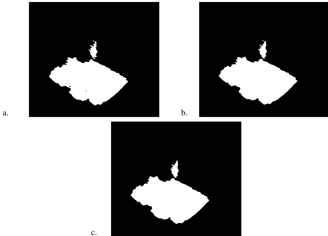
Figure 3.4: a. Rough segmentation output from active contour algorithm, b. Segmentation after morphological closing and hole filling, c. Segmentation after morphological opening.
