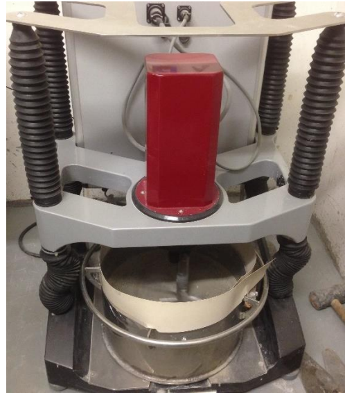
Figure 4.1. Planetary rheometer used to evaluate the fresh state properties.
