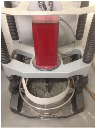
Figure 3.5. Planetary rheometer used to evaluate the fresh state properties, an example for C-161-0.37c-0.21f.
