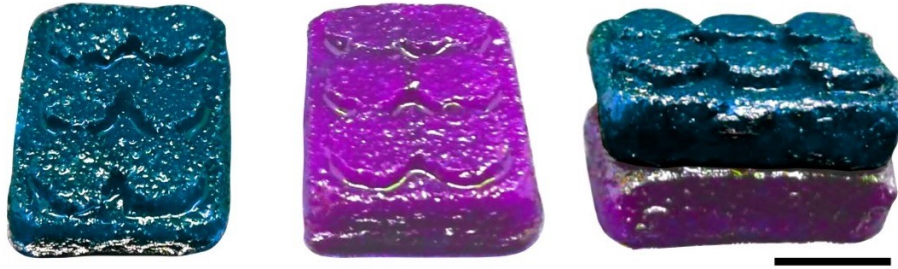
Supplementary Fig. 4.1: Classic 3x2 Lego TM block design. Two blocks were made from decellularized apple hypanthium tissue and were stained with Congo Red (magenta) and Calcofluor White (cyan). Scale = 1.5 cm.
