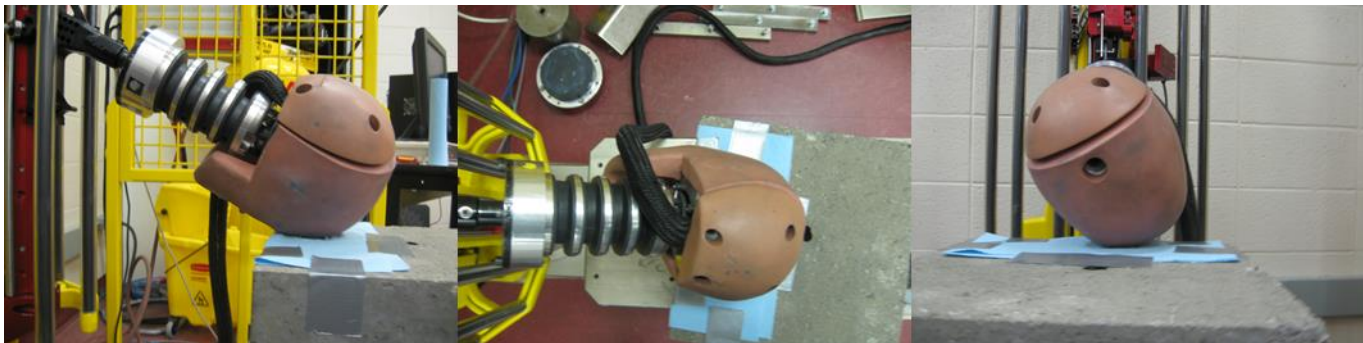
Figure 3. Hybrid III physical reconstruction of case 17.
