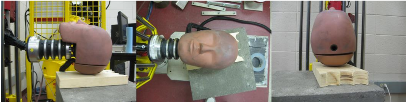
Figure 5. Hybrid III physical reconstruction of case 13.
