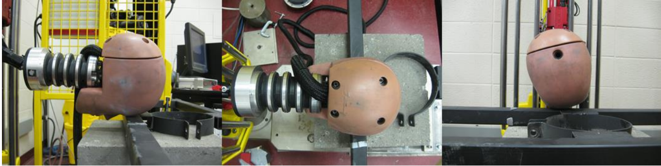
Figure 3. Hybrid III physical reconstruction of case 20.
