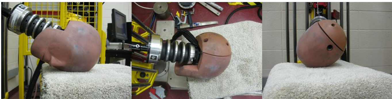
Figure 2. Physical reconstruction using a Hybrid III headform and neckform for a fall onto a carpet with underlay covering a concrete anvil
