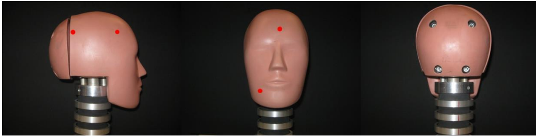
Figure 7. Parietal lobe SDH impact locations on the Hybrid III
