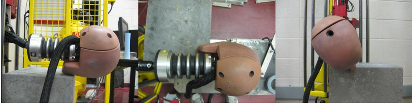
Figure 3. Hybrid III physical reconstruction of case 19.
