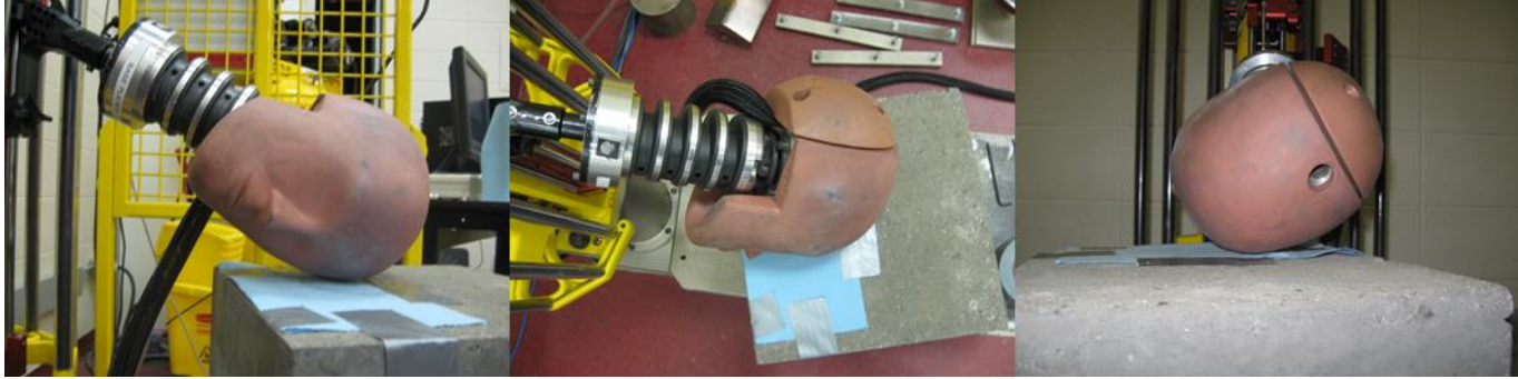
Figure 5. Hybrid III physical reconstruction of case 12
