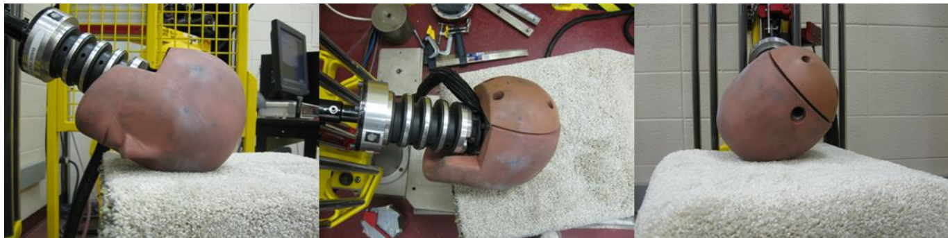
Figure 4. Hybrid III physical reconstruction of case 6.
