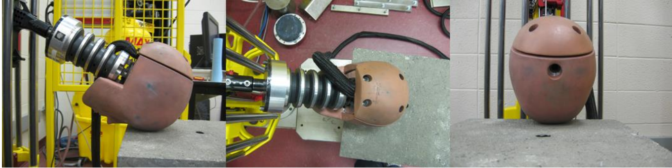
Figure 3. Hybrid III physical reconstruction of case 16.
