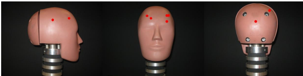
Figure 6. Frontal lobe SDH impact locations on the Hybrid III
