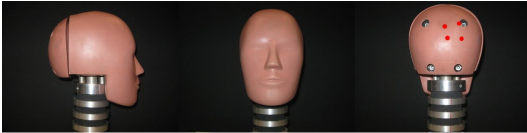
Figure 8. Occipital lobe SDH impact locations on the Hybrid III
