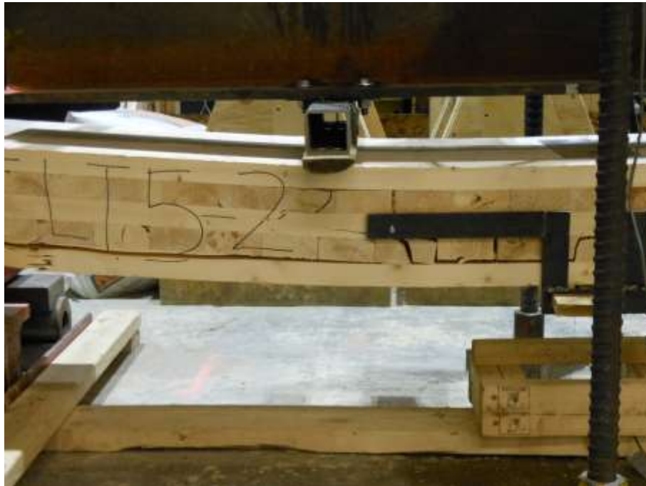
Figure A1.10: Development of Rolling Shear Post Flexural Failure in CLT5-2
