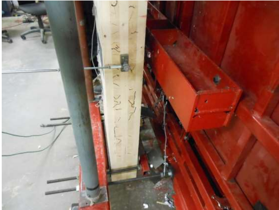
(a) Rolling Shear on Lower Right Side Following Light Flexural Failure
