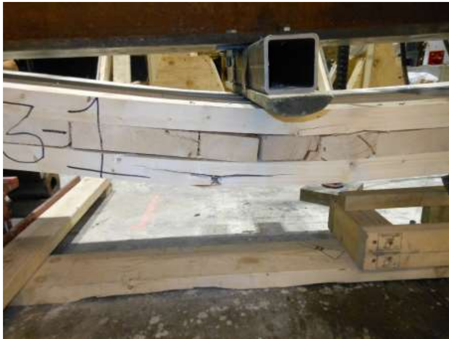
Figure A1.2: Flexural Failure in Tension Laminate and Rolling Shear in Transverse Laminate in CLT3-1
