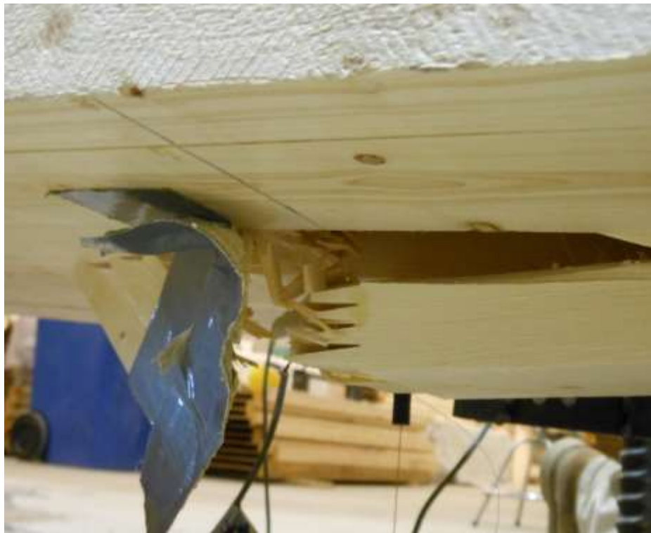
Figure 4.3: Shearing of Finger Joints in Tension Laminates
