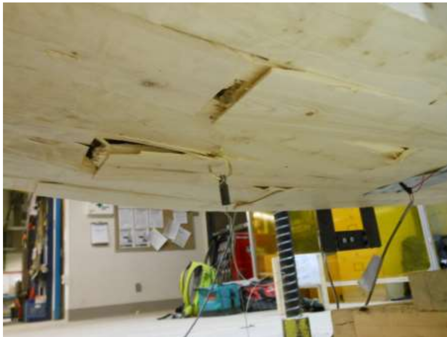
Figure A1.6: Flexural Failure along Finger Joints in CLT3-3
