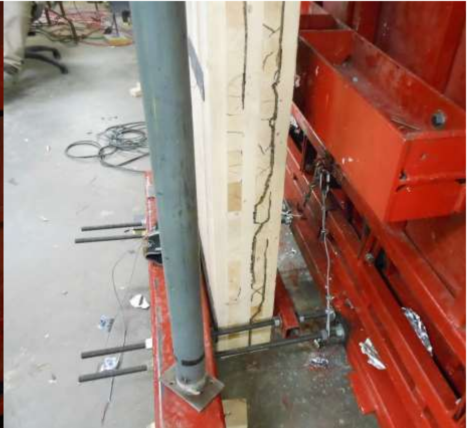
(b) Rolling Shear on Lower Right Side of Panel
