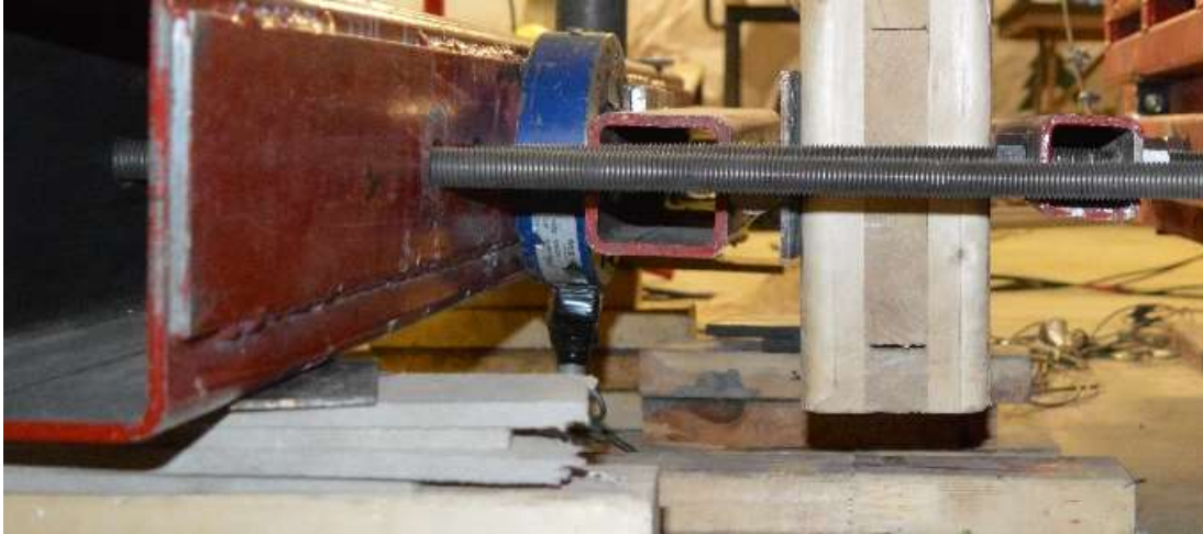
(a) Support with load cell
