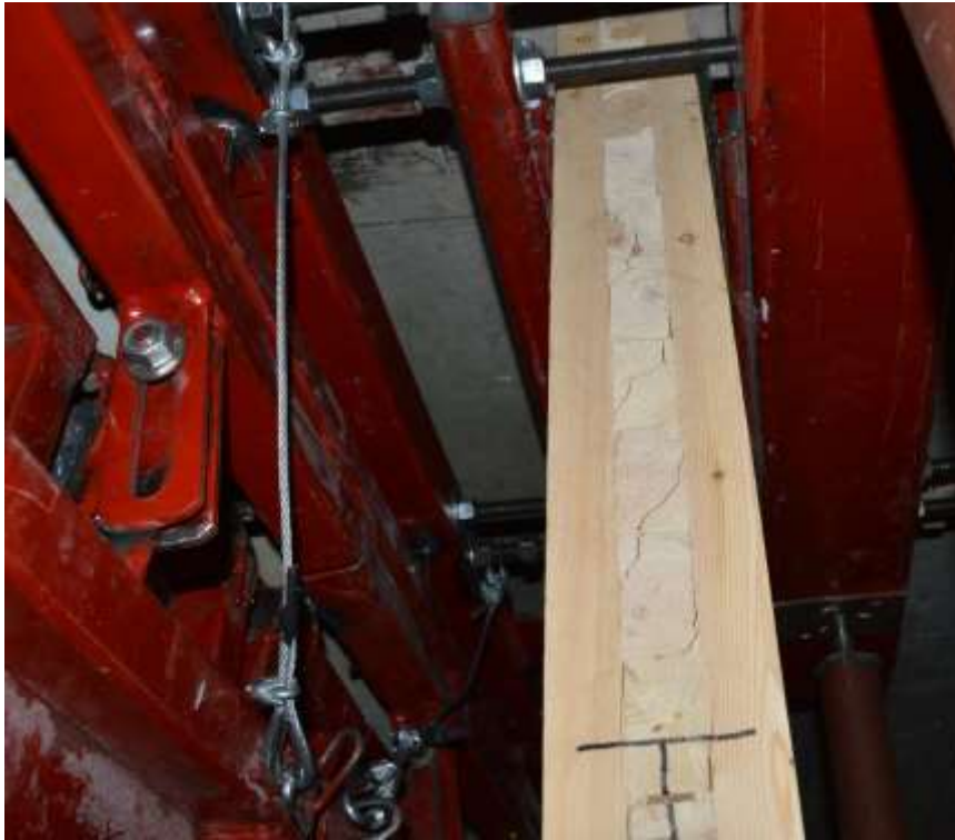
(a) Rolling Shear on upper Left Side
