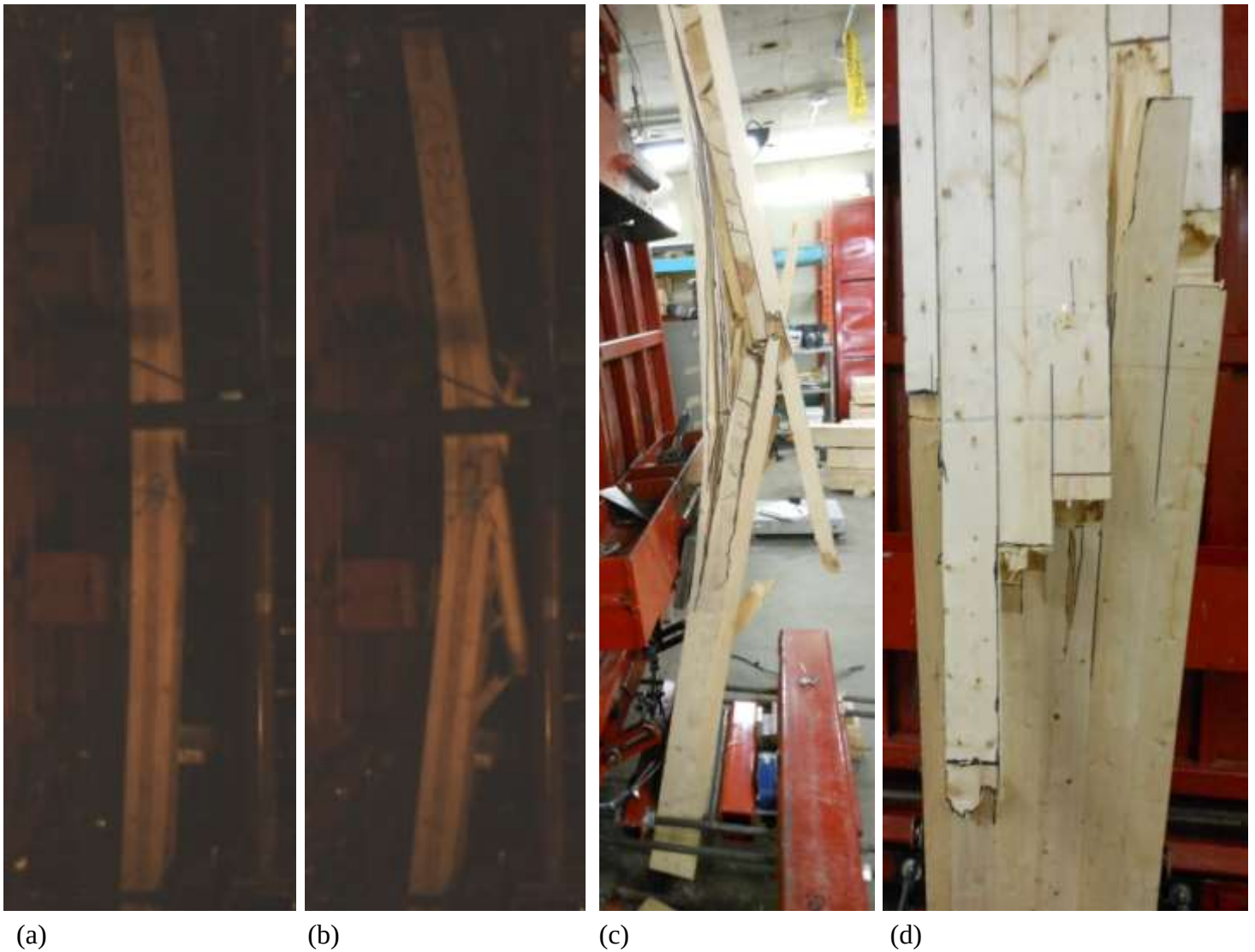
Figure 4.10: Flexural failure (CLT3-5.1): (a) maximum displacement prior to failure; (b) flexural failure in the tension laminates; (c) failed panel post-test; (d) flexural failure through a series of finger joints
