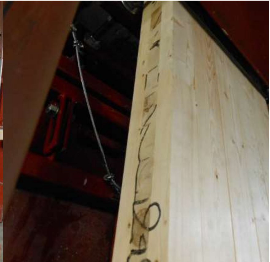
(b) Rolling Shear at Upper Left Side
