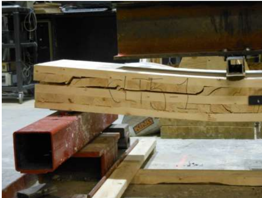
Figure A1.8: Development of Rolling Shear Post Flexural Failure in CLT5-1
