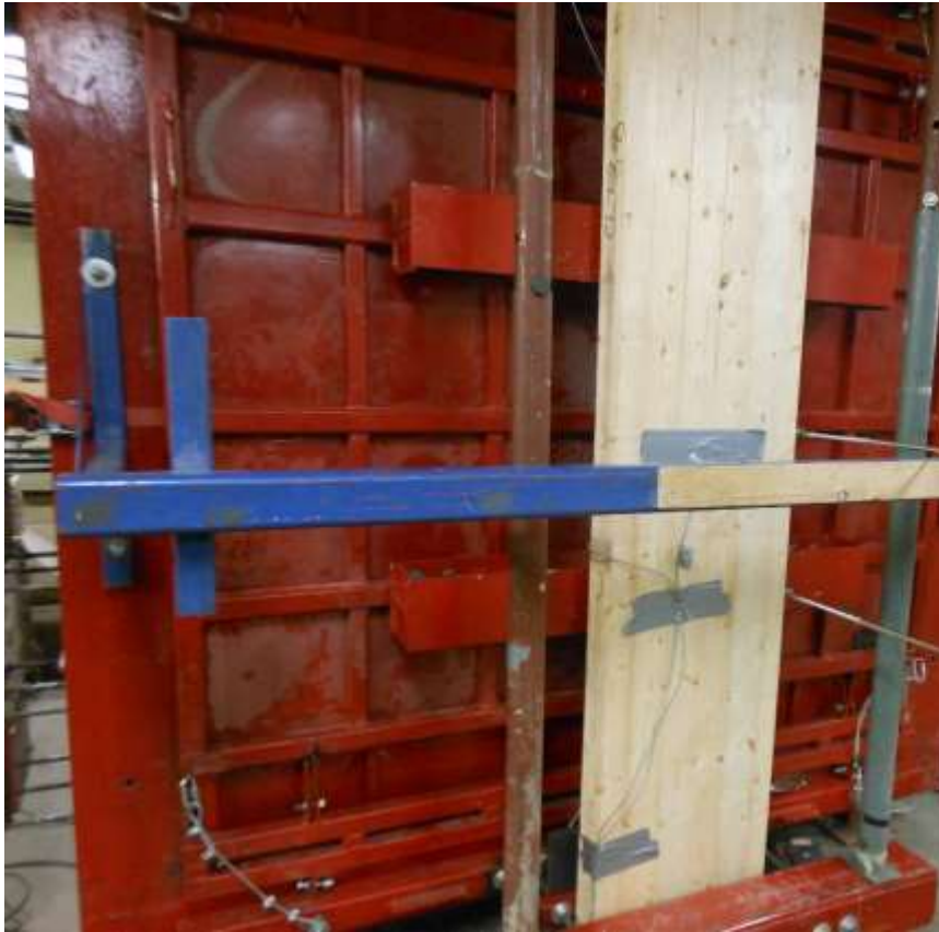
(a) No Flexural Damage Post Test
