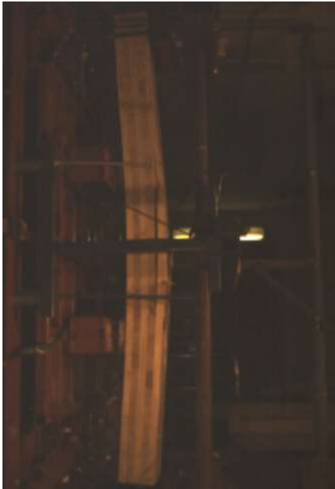
(a) Start of Flexural Failure – Left Side
