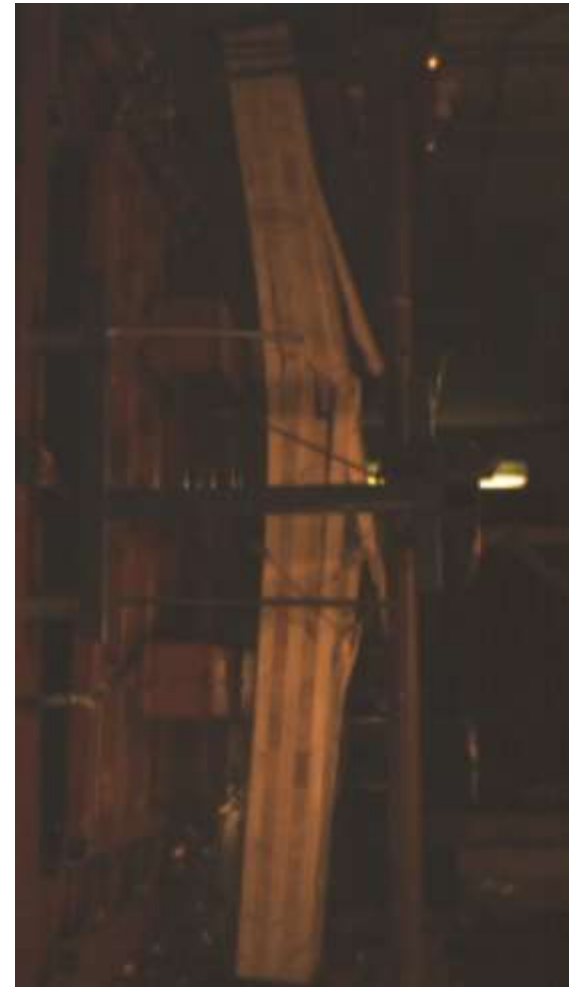
(b) Full Flexural Failure – Left Side
