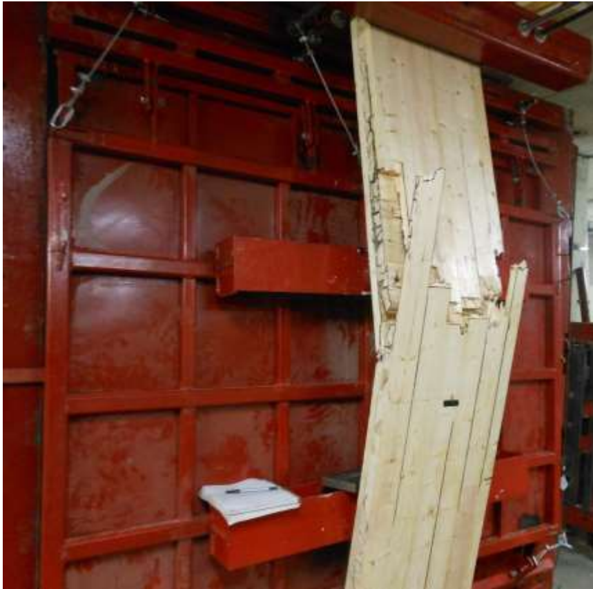
(a) Flexural Failure – Front Face
