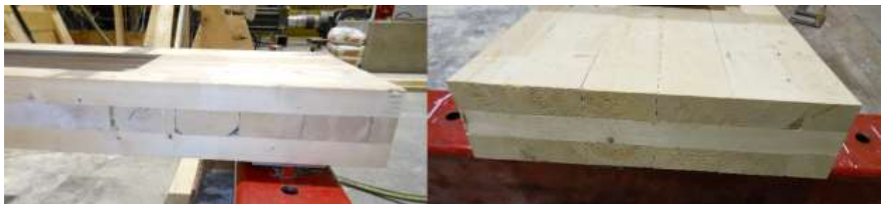
Figure 1.1: Typical 3-ply CLT Panel
