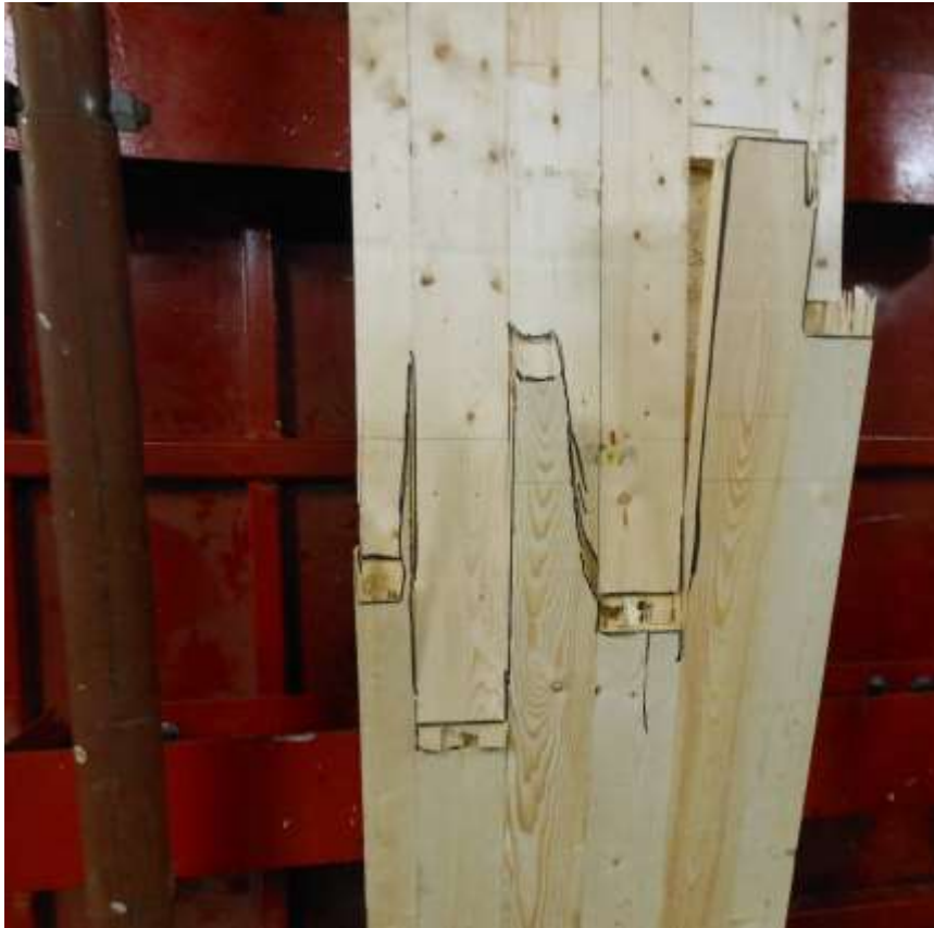
(a) Flexural Failure along Finger Joints
