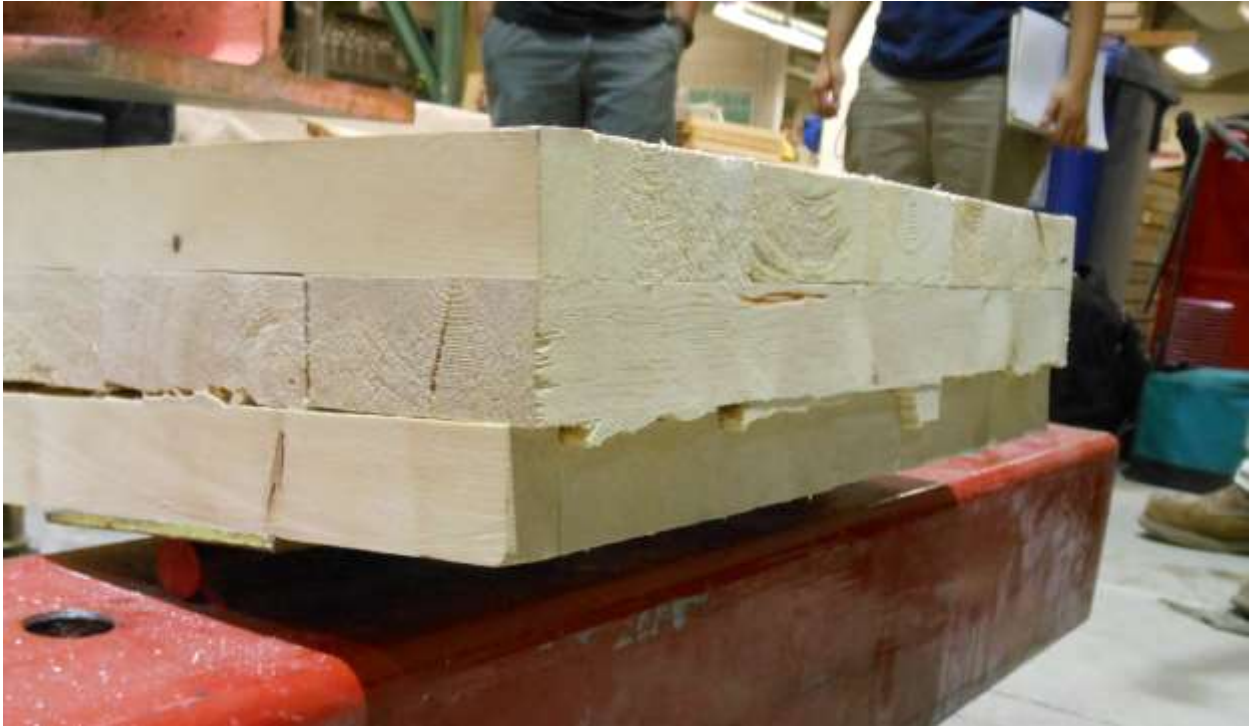
Figure 4.4: Longitudinal Shear in Tension Laminates
