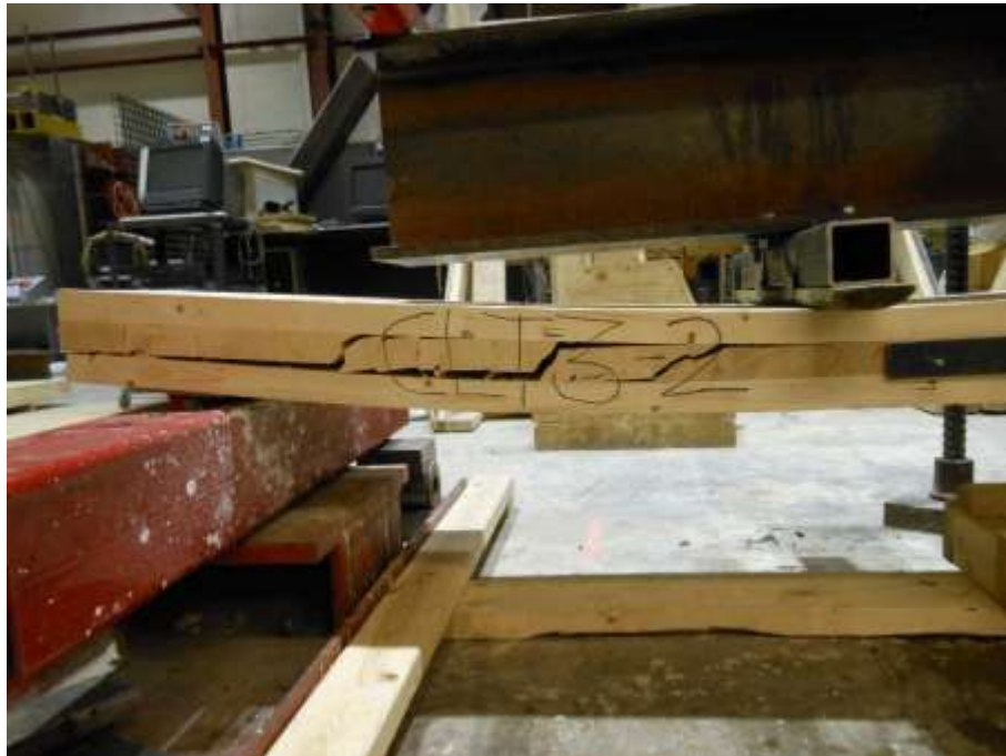
Figure A1.4: Rolling Shear Developed in Transverse Laminate in CLT3-2
