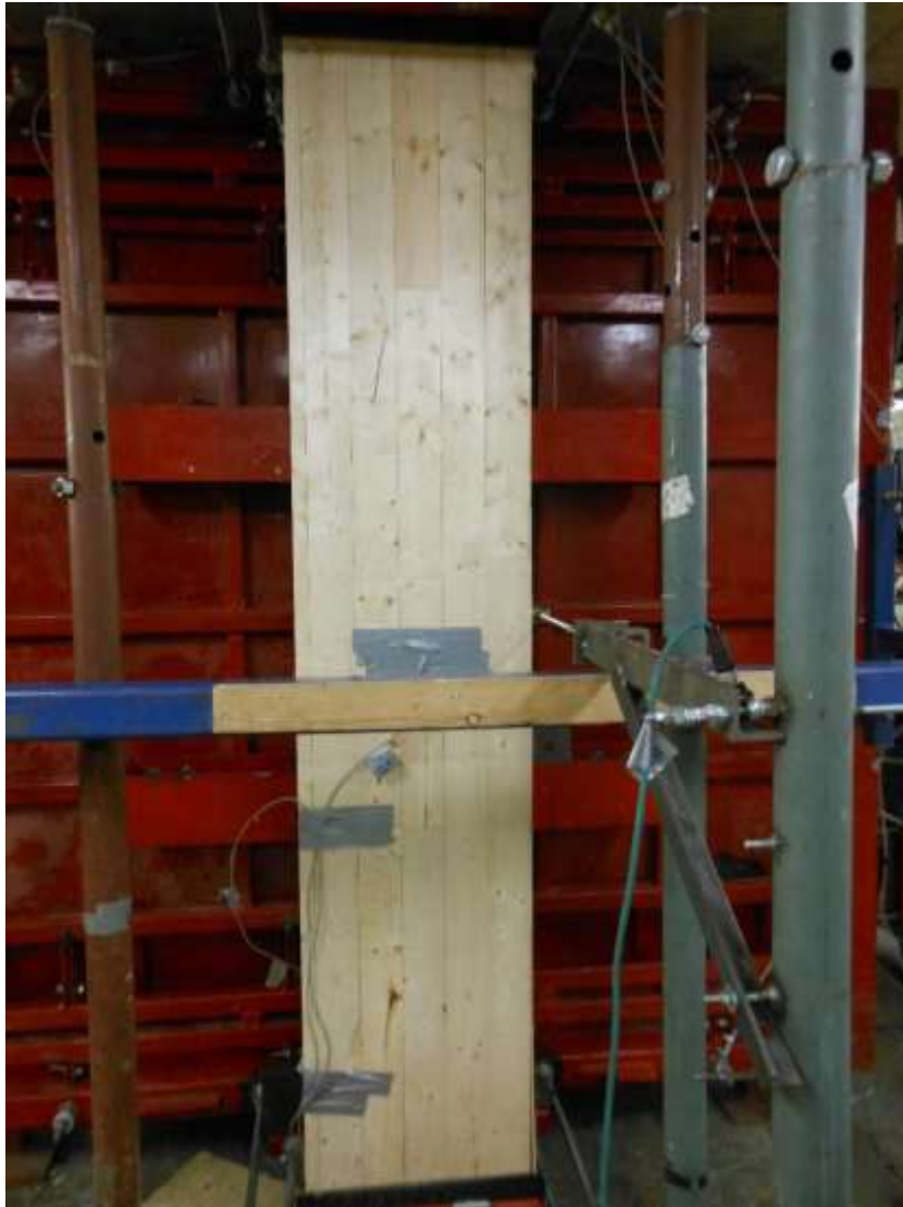
(a) No Significant Flexural Damage Post Test – Front Face
