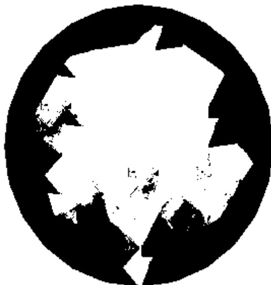
Figure 3.22 – Additional example of superimposed and filtered collection of 500 antenna shapes, similar to the previous figure only with the electrical size of the antennas equal to ka = 0.40 (circular antenna shapes are used)
