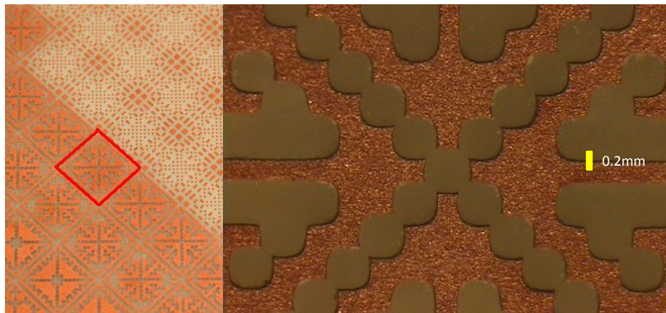
Figure 5.35 – Magnified view of a problem-free reflectarray element, achieved due to the vertex-fixing approach
