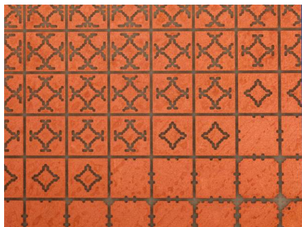
Figure 5.33 – High resolution and detailed photographs of similarity-optimized fragmented reflectarray with photo courtesy of Communications Research Centre Canada (CRC), Photographer: John Brebner.
