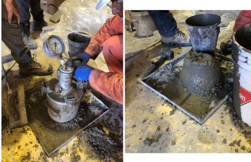
Fig. 3.4: Left: air content test, Right: slump test
