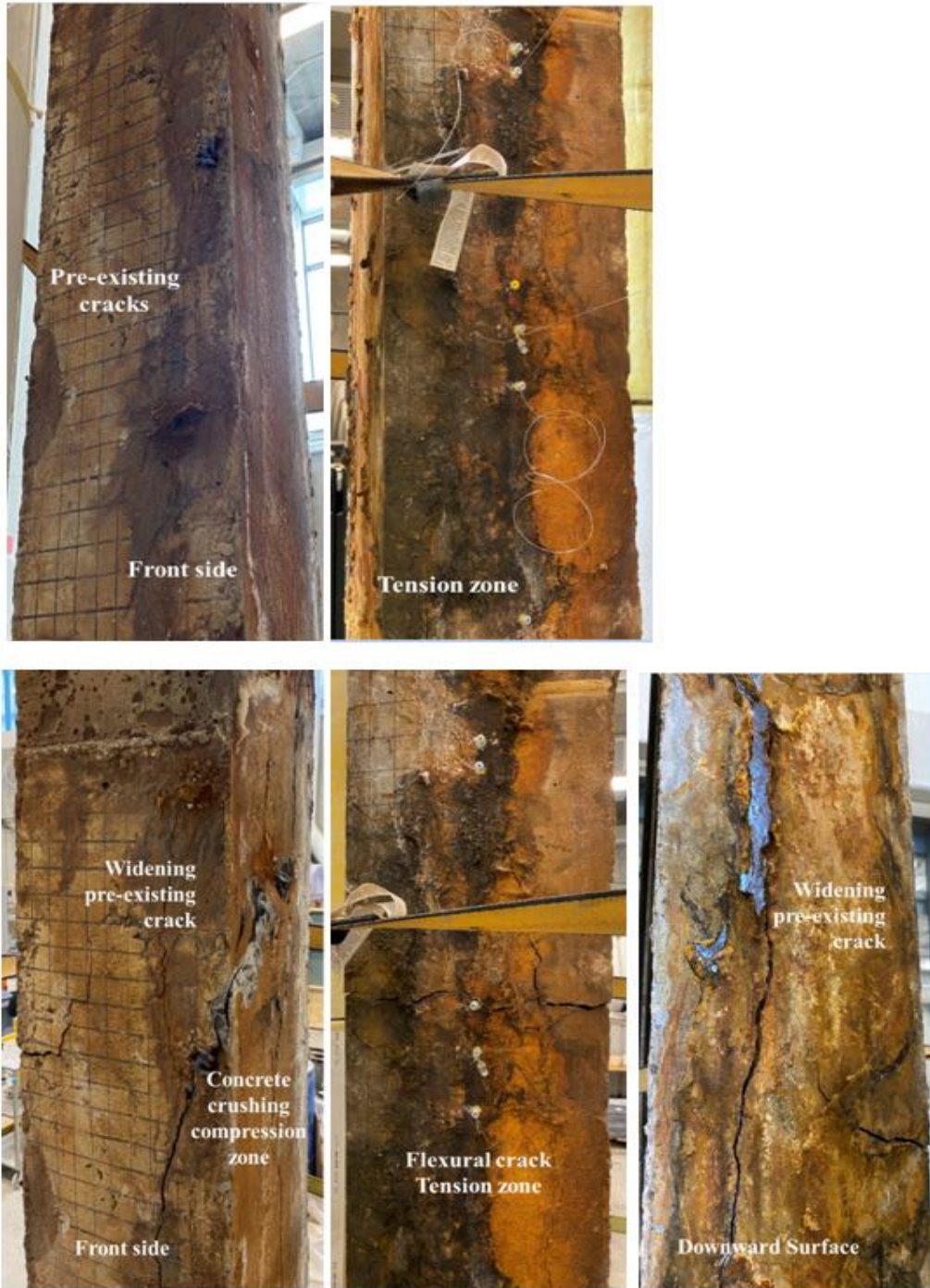
Fig. 5.7: Failure mechanism of specimen C-E-R1
