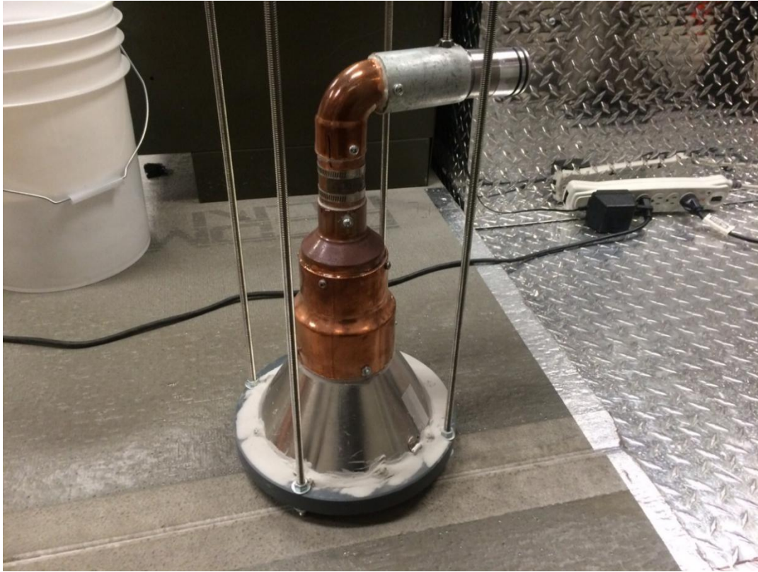
Figure A.9. View of the large elbow. Approximate height of 0.42 m.
