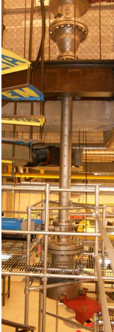
Figure A.1. Vertical profile of the 2.94 m fluidization column.
