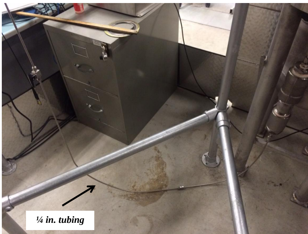
Figure A.4. View of the initial section of the 0.006 m (1/4 in.) pneumatic convey line for fines.
