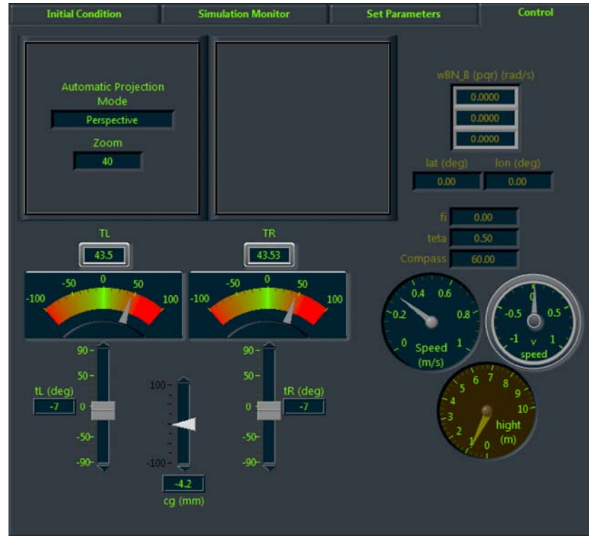
Fig. 6.68: A sample of control and display unit when the AUV at a depth of 1m.
