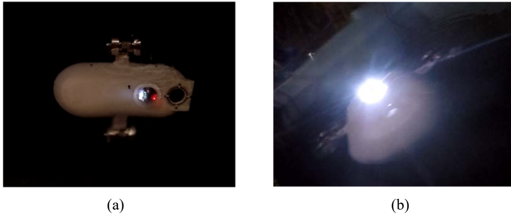
Fig. 4.16: (a) View of the AUV at night, (b) LEDs performance with maximum power.
