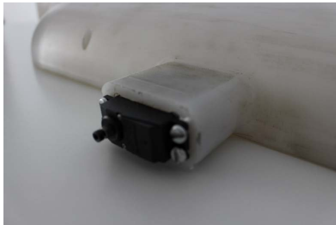
Fig. 3.27: The servo motor in the dolly blocks.
