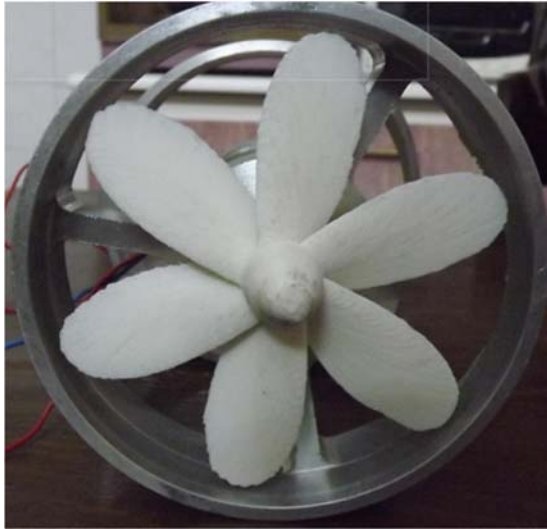
Fig. 3.26: The propellers in the thruster.
