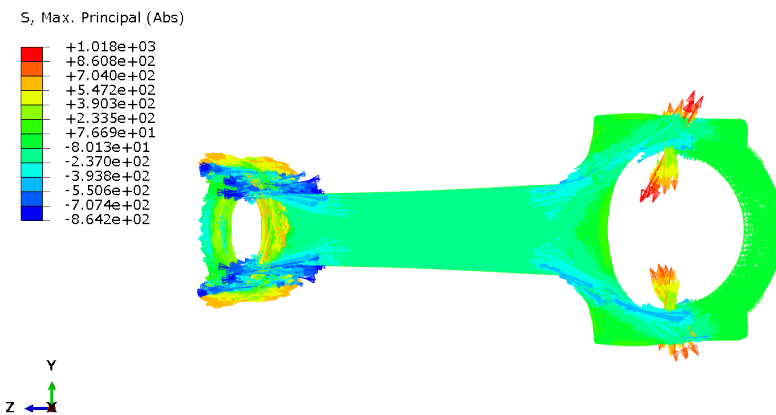
(b) Principal stress vectors (isometric view)
