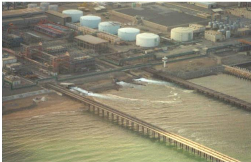
Figure 2.1. Surface discharge of the Al-Ghubrah desalination plant, the largest such facility in Oman (Source: H.H. Al-Barwani).
