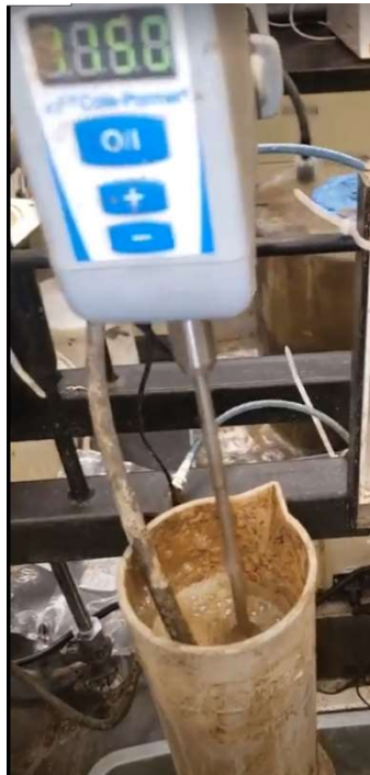
Figure Appendix 11-17: Foam control in the semi-continuous stripping column.
