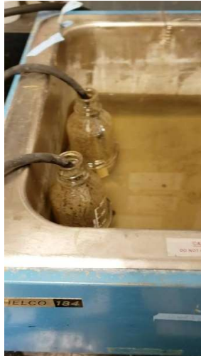
Figure Appendix 11-3: Ammonia stripping bottle in water bath for Phases I and II.
