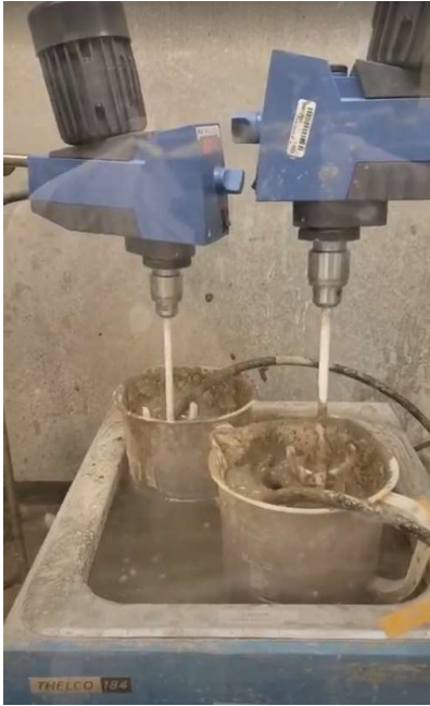
Figure Appendix 11-16: Ammonia stripping of 2 Liters per reactor using renewable natural gas conducted in fume hood. Mixers are only used for foam control in the headspace.
