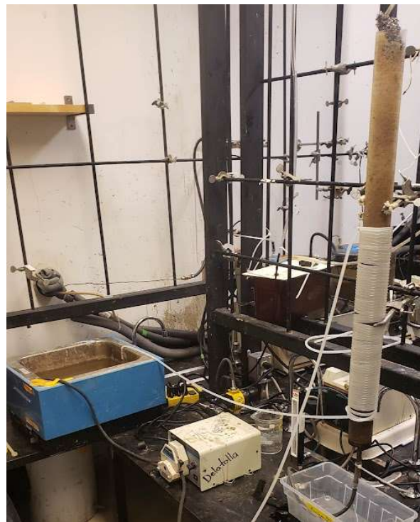
Figure Appendix 11-15: Ammonia stripping column in the semi-continuous experiment in Phase IV (air stripping).
