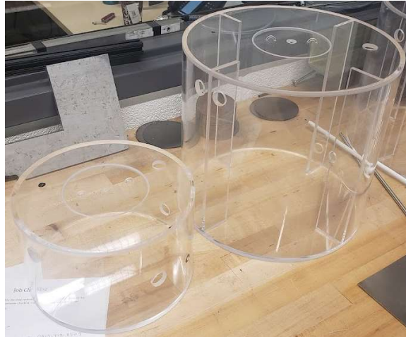
Figure 3-8: Hydrolyzer CSTR (5 liters) and anaerobic digester CSTR (15 Liters).
