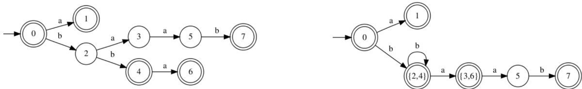
Figure 2.4: State-merging DFA induction starting from a prefix-tree acceptor. [25].
