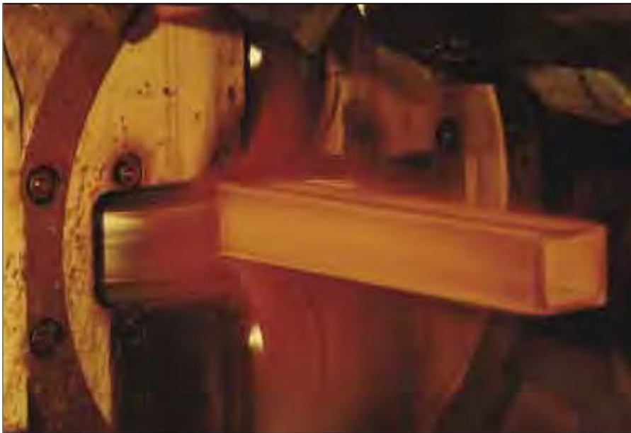
Fig. 1.10: HSS passing through the shaping rollers (Photo from VMTubes 2008)
