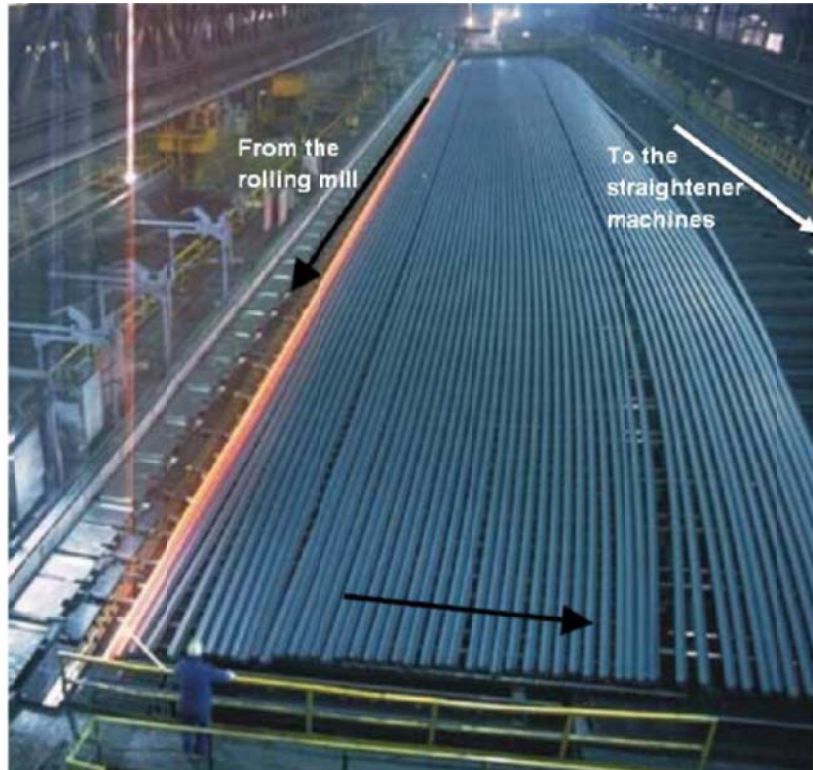
Fig. 1.5: Cooling bed and straightener machines for rail sections (Photo from Espinoza 2007)
