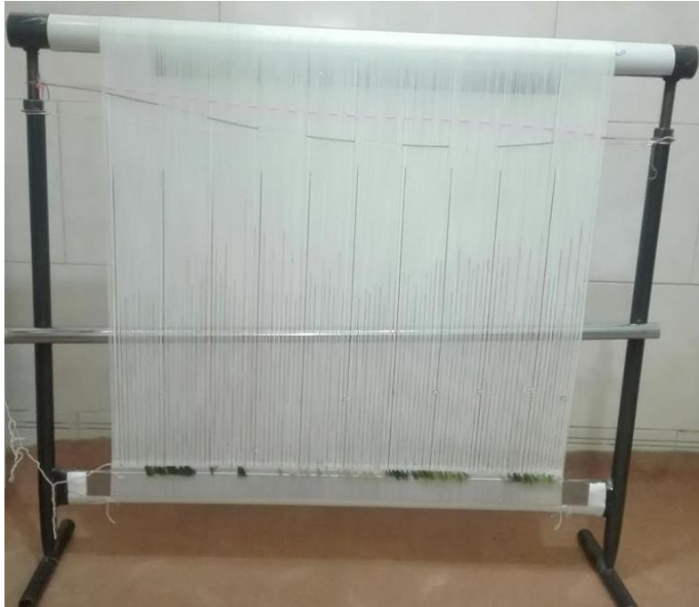
Figure 17 Blank loom, ready to be woven on Toranjomehrab 2017 Photo credit Ghazaleh Jerban
