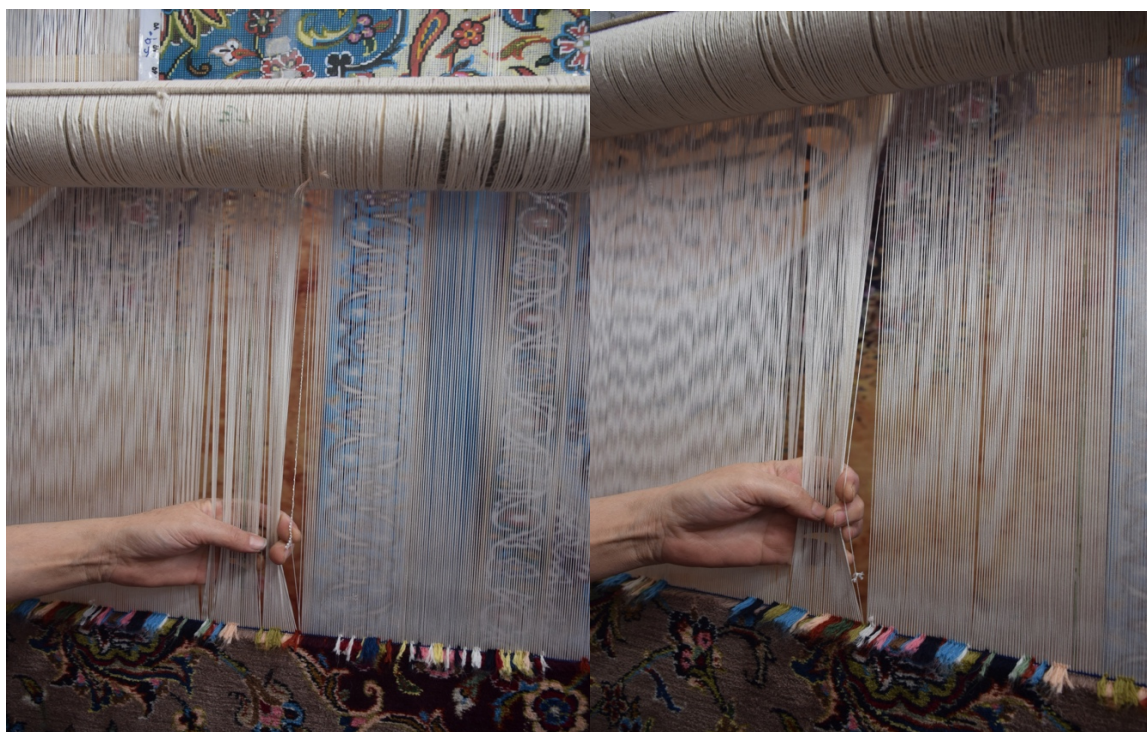
Figure 20 Two examples of wraps being broken which should be fixed by a skilled weaver. Tornajomehrab workshop, 2017 Photo credit Ghazaleh Jerban
