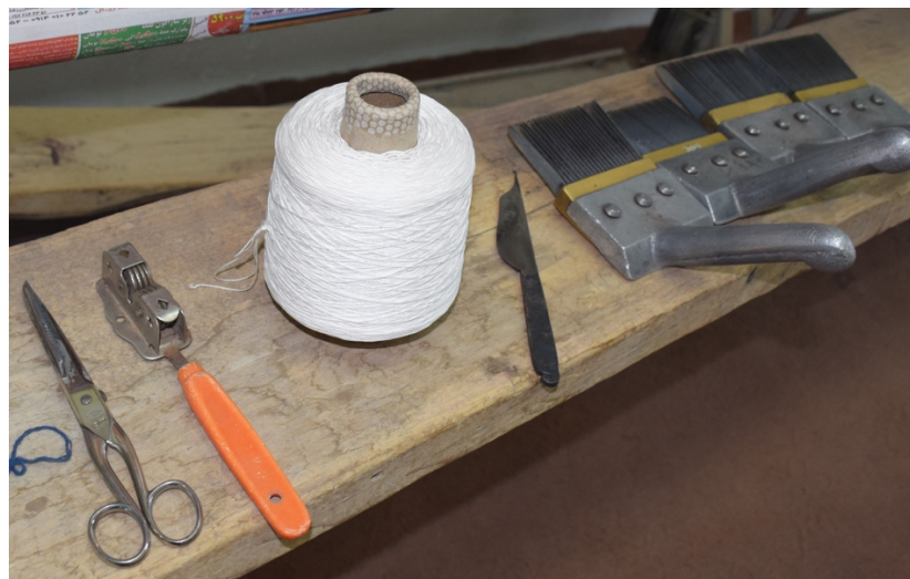
Figure 19 From left to right: Special scissors, sharpener, fibre, hook, comb beater Photo credit Ghazaleh Jerban
