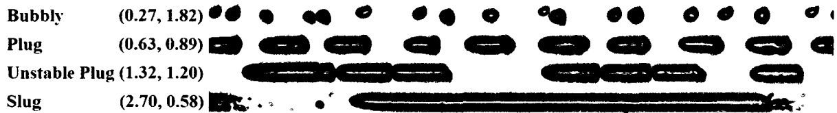
Figure 2.9 Flow patterns observed for the given gas and liquid velocity, (U_D, U_C) , at a location 27 to 45 channel diameters downstream of the T-junction.
