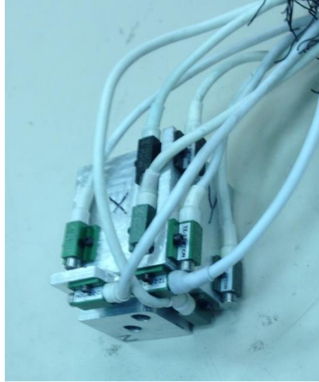
Figure 2: Orthogonally positioned 3-3-3-2 accelerometer array.
