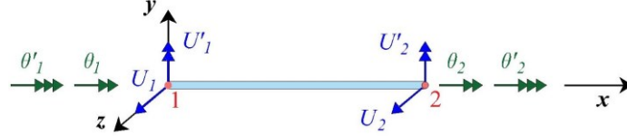
Fig. 3.2 Degrees of freedom of the BG element employed in the LTB-UO program
