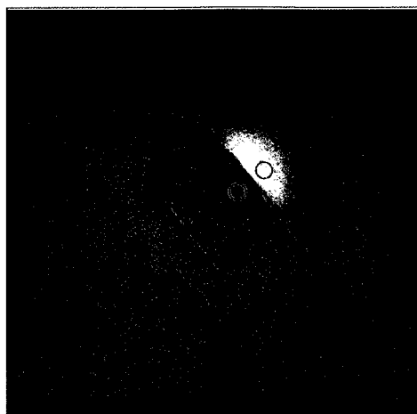
Figure 5.10: The ice-water interface. Ice is observed on the left side of the image and water is observed on the right. The blue and red circles correspond to areas used to obtain CARS spectra for the water and ice.
