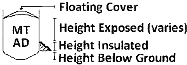
Figure 4.12 Anaerobic digester design schematic
