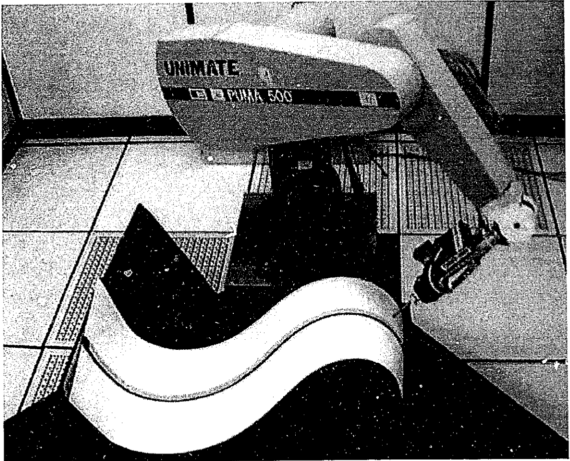
Figure 5.20: Photograph showing the PUMA robot executing the follow edge skill.
