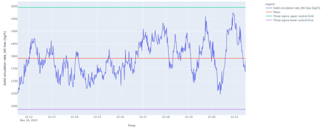
Figure 76. Timeseries graphs for solid circulation rate at the 0.05 m weir opening height condition (third repeat).
