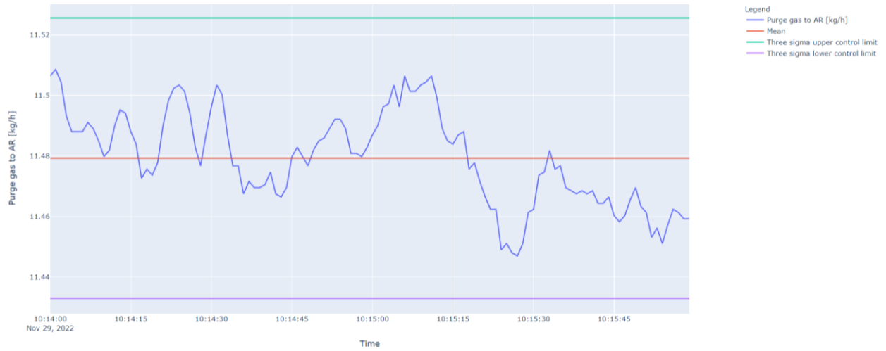
Figure 97. Timeseries graphs fate of the amount of AR/FR purge gas that remained in the air reactor at the 0.125 m weir opening height condition (first repeat).
