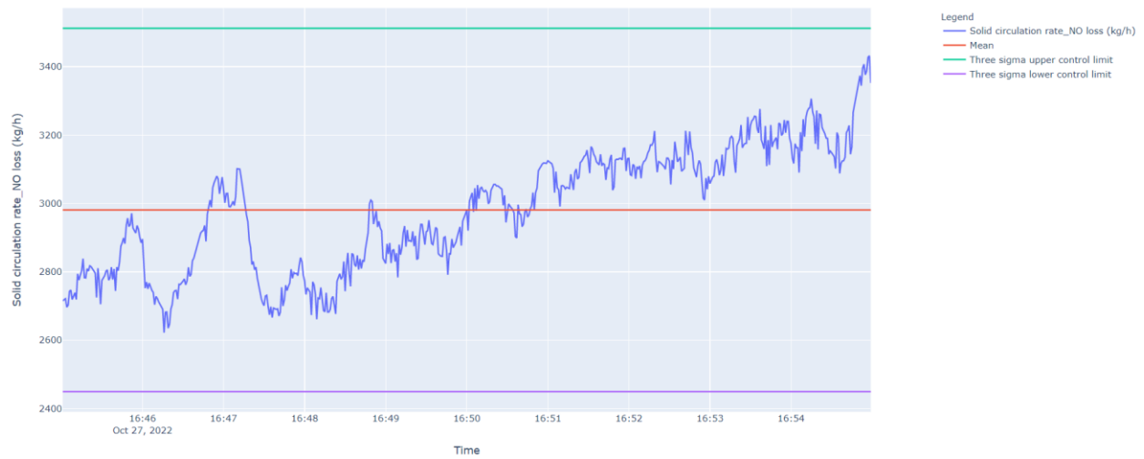
Figure 31. Timeseries graphs for solid circulation rate at the base case condition (second repeat).
