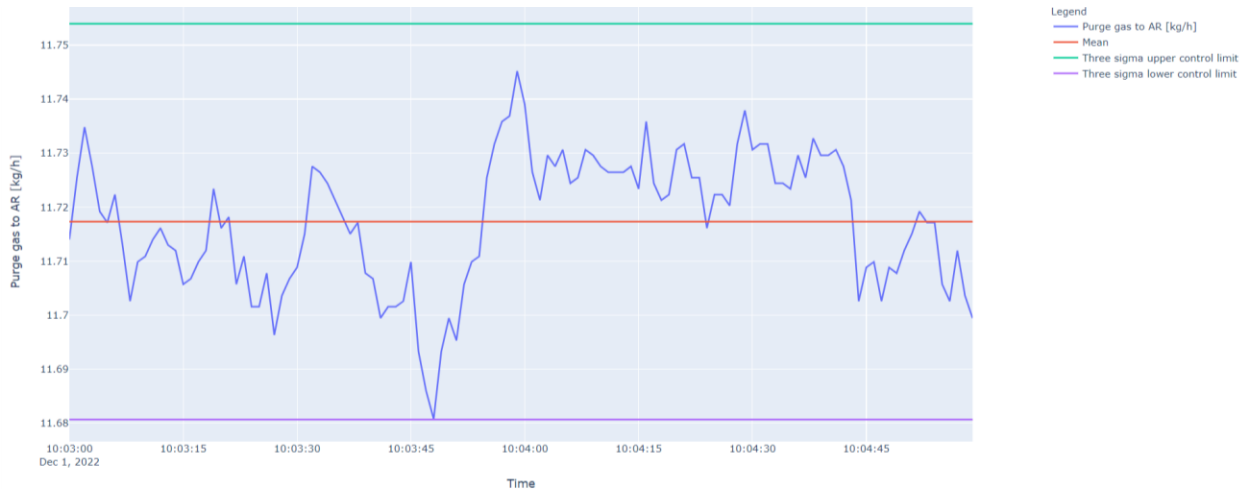
Figure 110. Timeseries graphs fate of the amount of AR/FR purge gas that remained in the air reactor at the 0.15 m weir opening height condition (first repeat).
