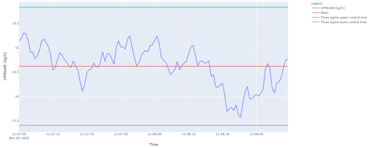
Figure 95. Timeseries graphs for fuel reactor to air reactor gas leakage at the 0.125 m weir opening height condition (first repeat).
