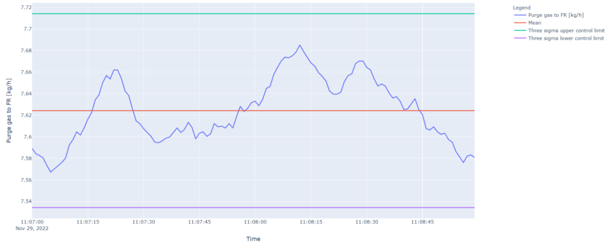
Figure 103. Timeseries graphs fate of the amount of FR/AR purge gas that remained in the fuel reactor at the 0.125 m weir opening height condition (first repeat).
