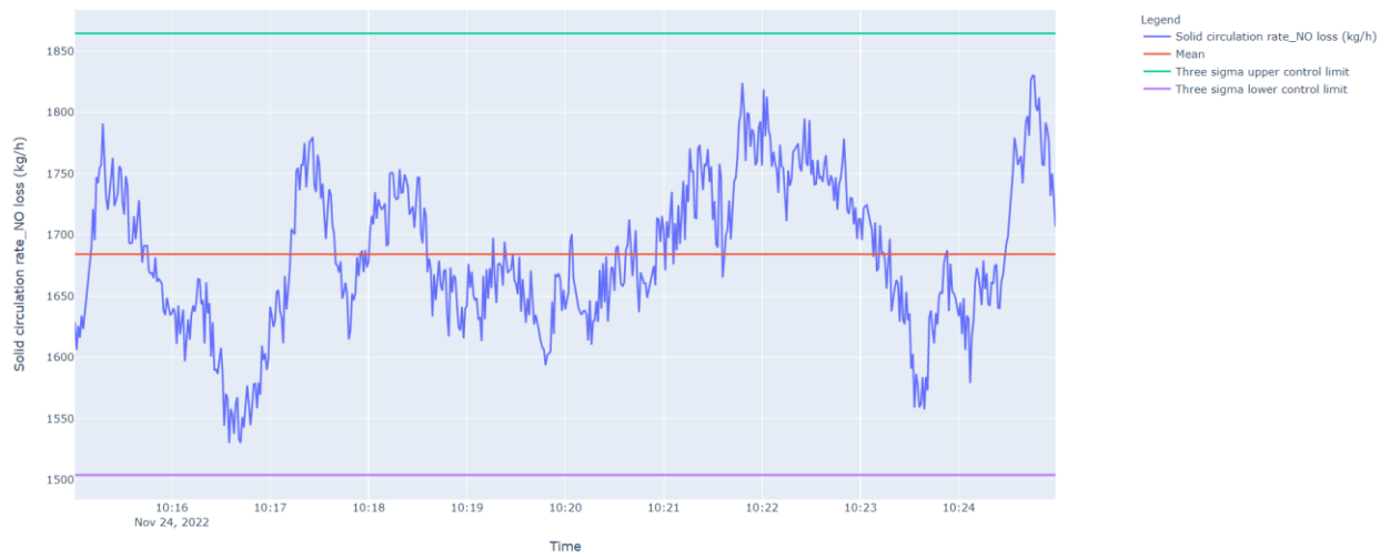
Figure 74. Timeseries graphs for solid circulation rate at the 0.05 m weir opening height condition (first repeat).
