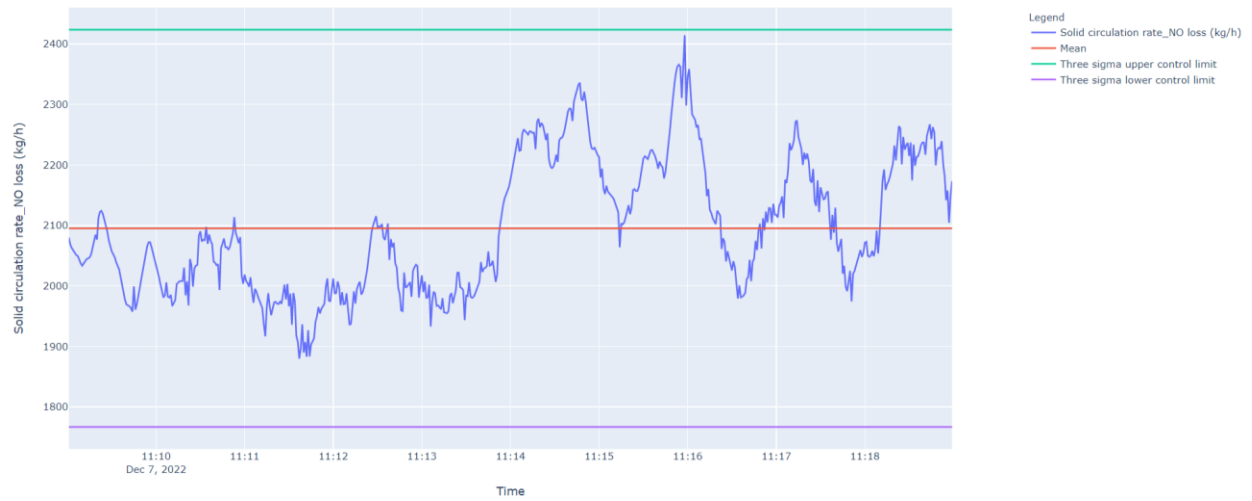
Figure 149. Timeseries graphs for solid circulation rate at the two AR/FR purge tuyere condition (third repeat).
