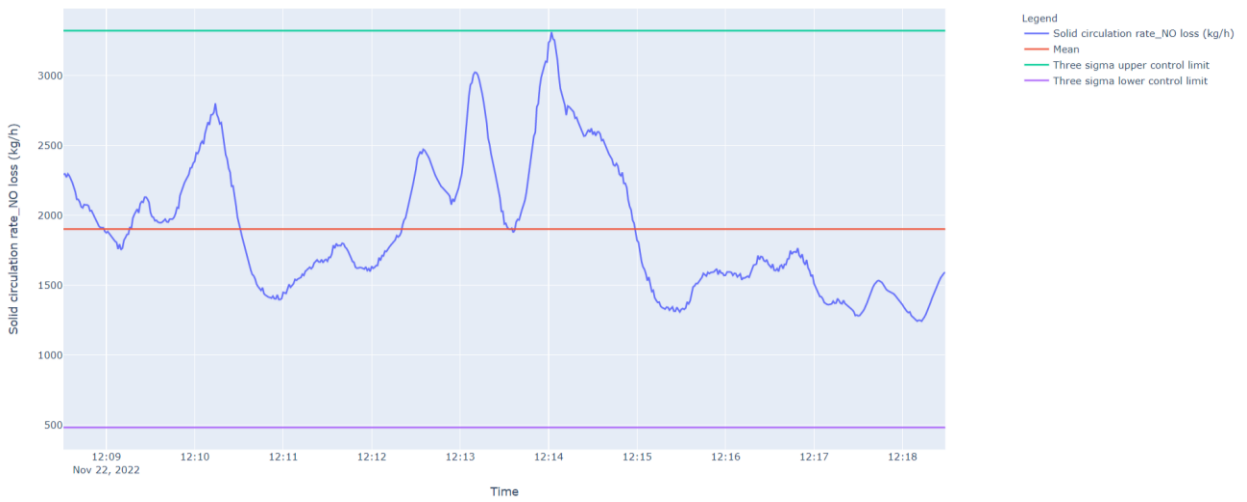
Figure 124. Timeseries graphs for solid circulation rate at the blank purge tuyere condition (second repeat).
