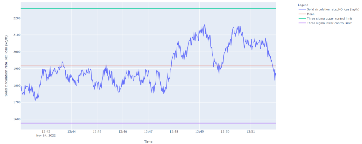
Figure 77. Timeseries graphs for solid circulation rate at the 0.05 m weir opening height condition (forth repeat).
