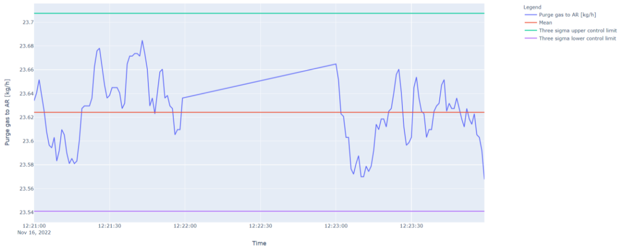
Figure 140. Timeseries graphs fate of the amount of AR/FR purge gas that remained in the air reactor at the vertical purge tuyere condition (second repeat).
