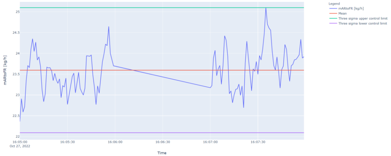
Figure 35. Timeseries graphs for air reactor to fuel reactor gas leakage at the base case condition (first repeat).
