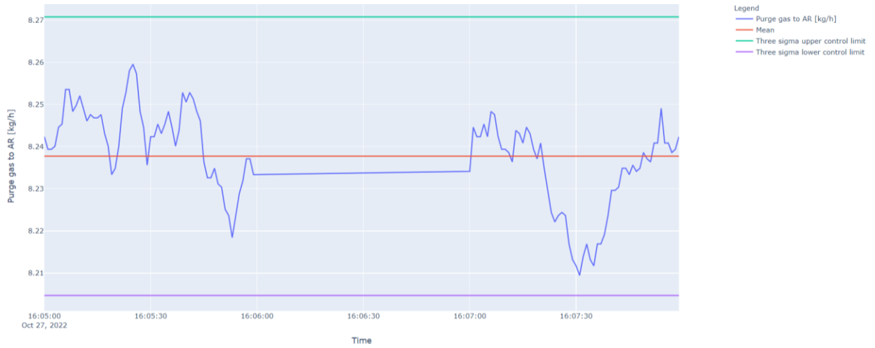
Figure 40. Timeseries graphs fate of the amount of AR/FR purge gas that remained in the air reactor at the base case condition (first repeat).
