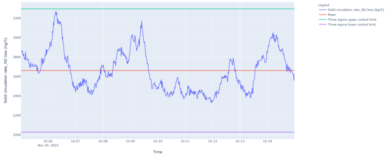
Figure 90. Timeseries graphs for solid circulation rate at the 0.125 m weir opening height condition (first repeat).
