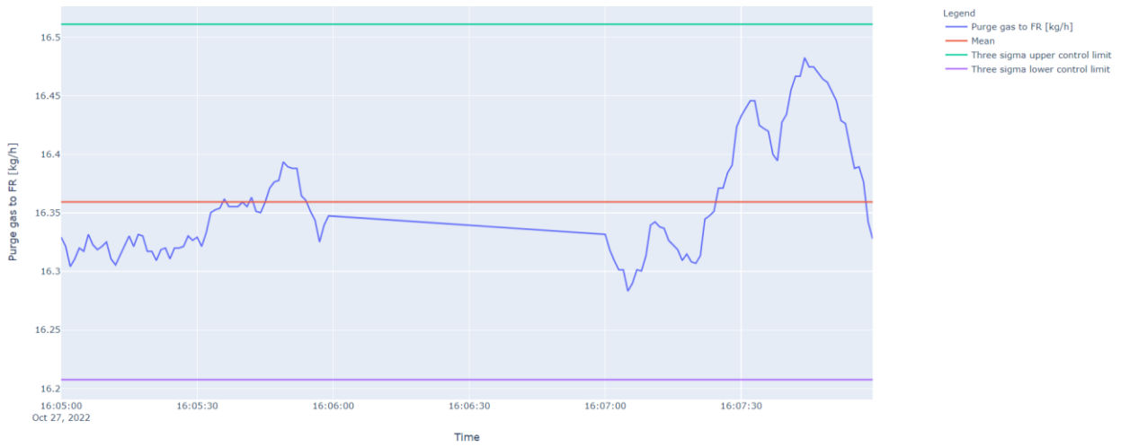
Figure 43. Timeseries graphs fate of the amount of AR/FR purge gas that moved to the fuel reactor at the base case condition (first repeat).
