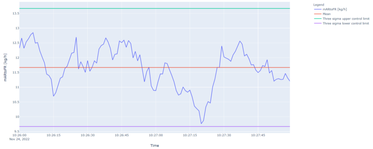
Figure 78. Timeseries graphs for air reactor to fuel reactor gas leakage at the 0.05 m weir opening height condition (first repeat).
