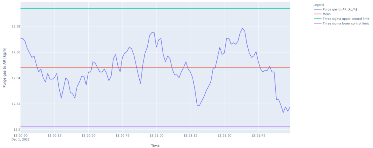
Figure 111. Timeseries graphs fate of the amount of AR/FR purge gas that remained in the air reactor at the 0.15 m weir opening height condition (second repeat).
