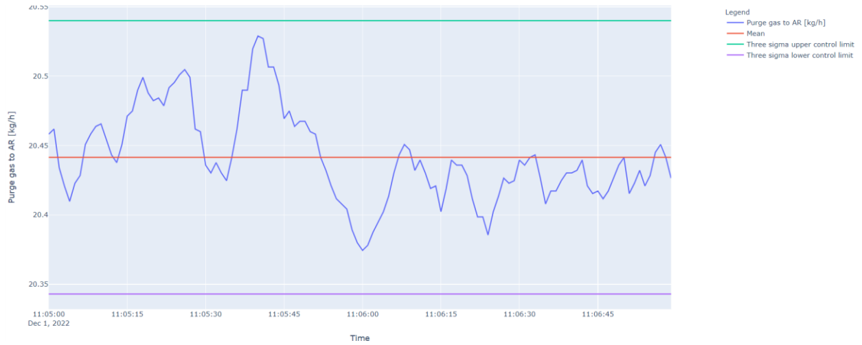
Figure 114. Timeseries graphs fate of the amount of FR/AR purge gas that moved to the air reactor at the 0.15 m weir opening height condition.
