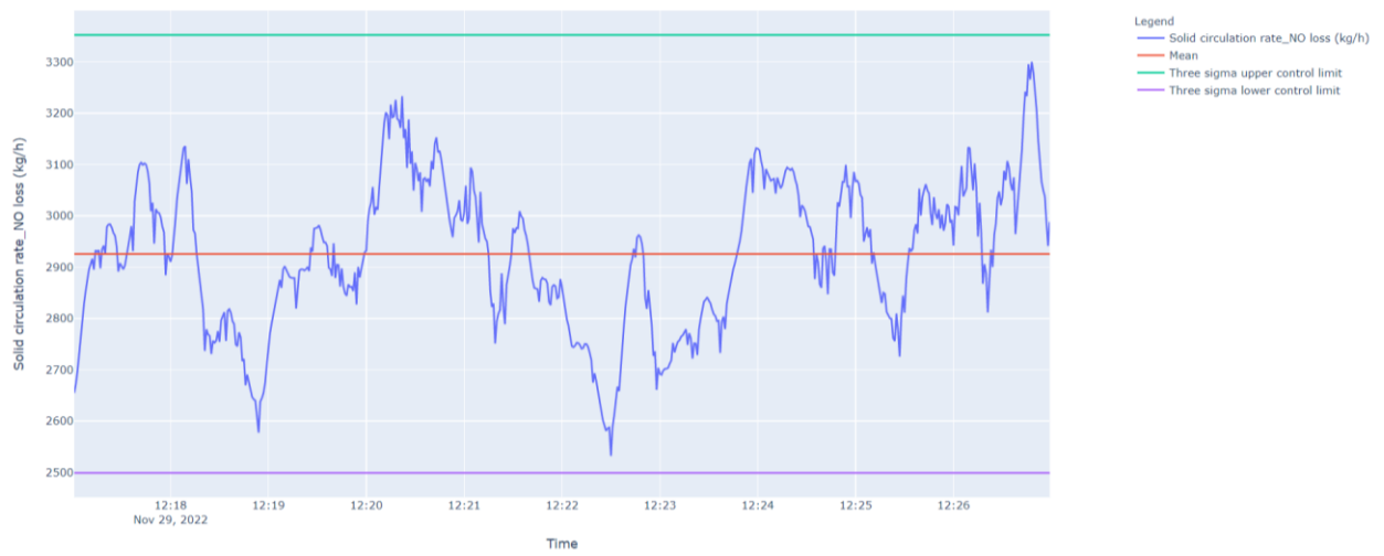
Figure 91. Timeseries graphs for solid circulation rate at the 0.125 m weir opening height condition (second repeat).
