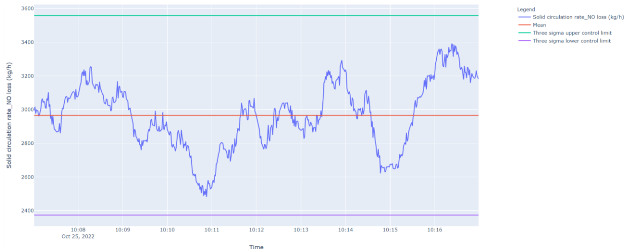
Figure 33. Timeseries graphs for solid circulation rate at the base case condition (fourth repeat).
