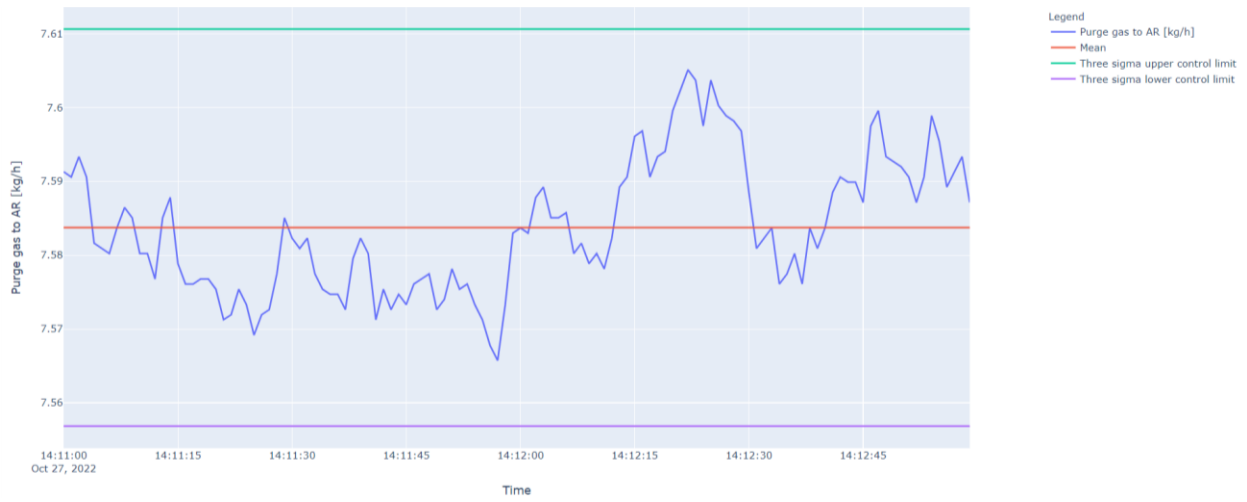
Figure 70. Timeseries graphs fate of the amount of AR/FR purge gas that remained in the air reactor at the 0.35 m bed height condition.
