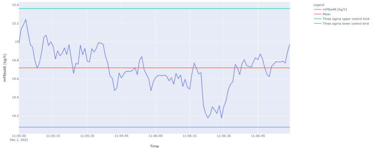
Figure 109. Timeseries graphs for fuel reactor to air reactor gas leakage at the 0.15 m weir opening height condition.
