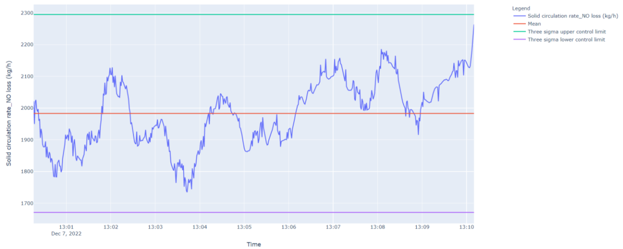
Figure 150. Timeseries graphs for solid circulation rate at the two AR/FR purge tuyere condition (fourth repeat).
