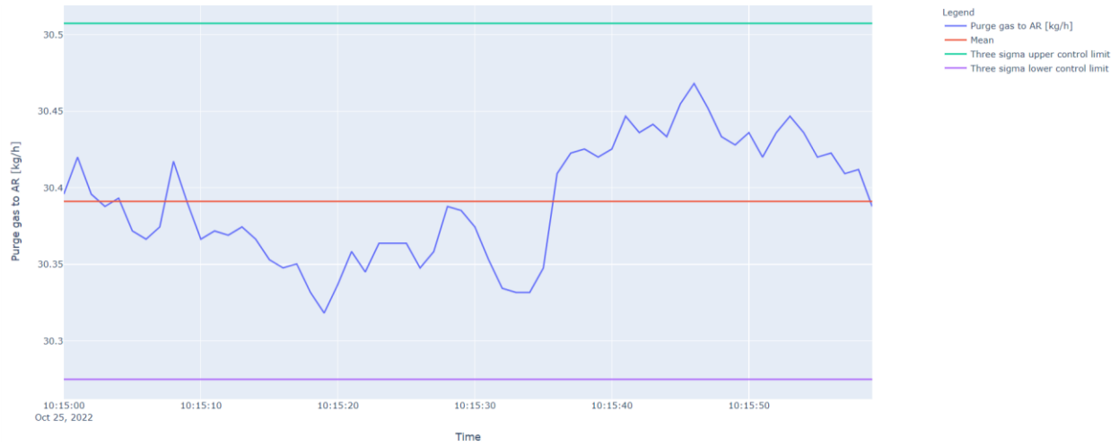
Figure 42. Timeseries graphs fate of the amount of AR/FR purge gas that remained in the air reactor at the base case condition (third repeat).
