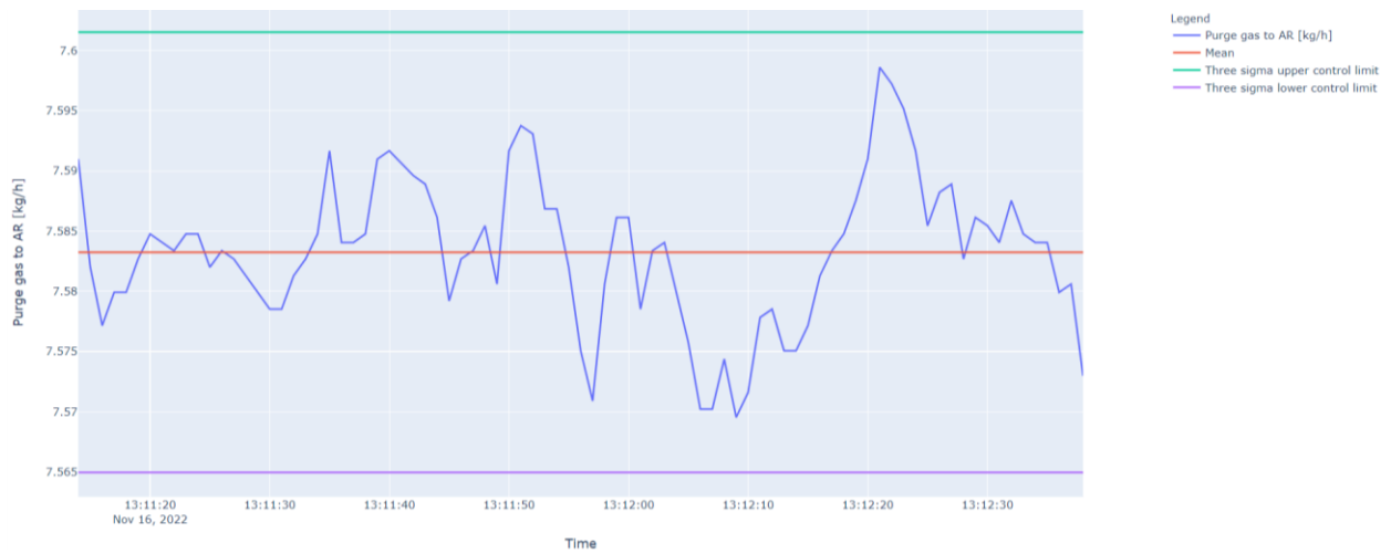
Figure 144. Timeseries graphs fate of the amount of FR/AR purge gas that moved to the air reactor at the vertical purge tuyere condition (second repeat).
