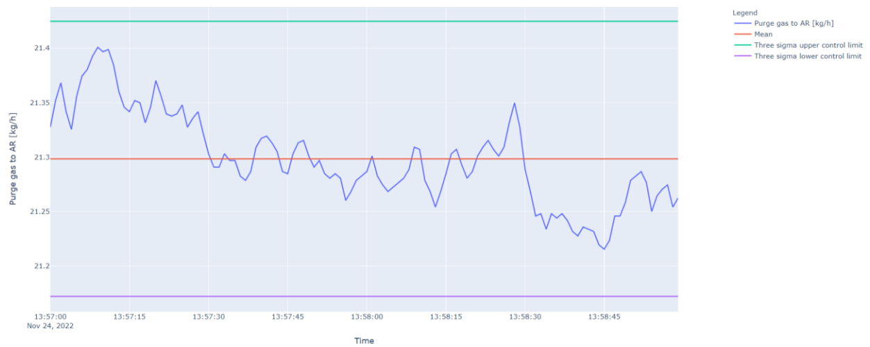
Figure 87. Timeseries graphs fate of the amount of FR/AR purge gas that moved to the air reactor at the 0.05 m weir opening height condition (second repeat).
