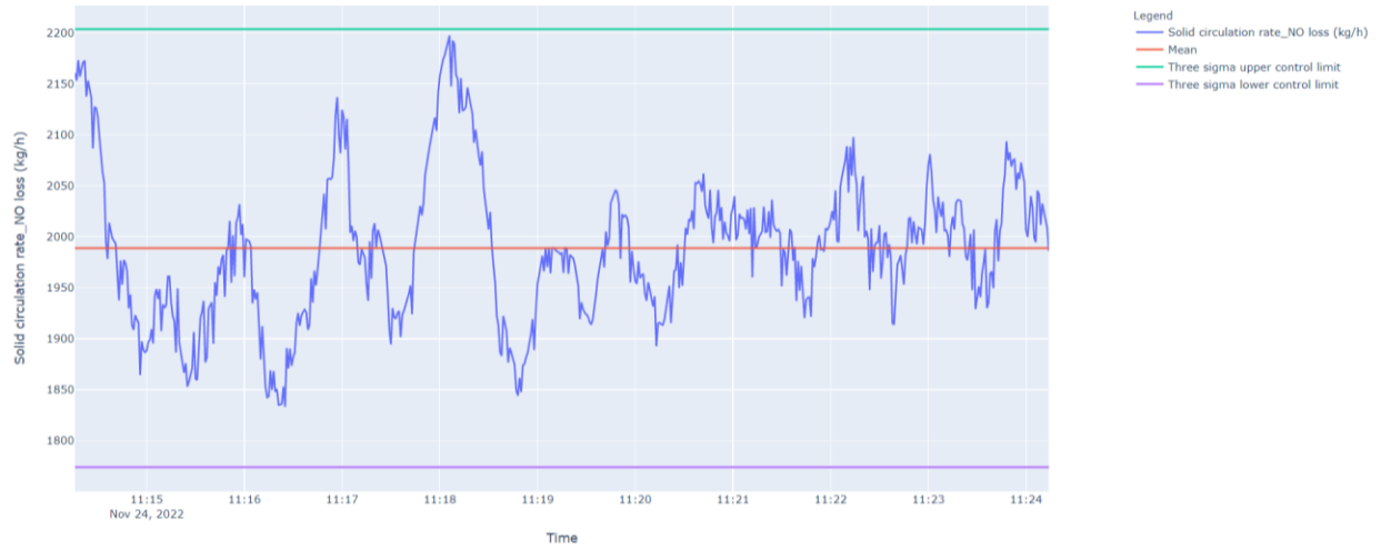
Figure 75. Timeseries graphs for solid circulation rate at the 0.05 m weir opening height condition (second repeat).
