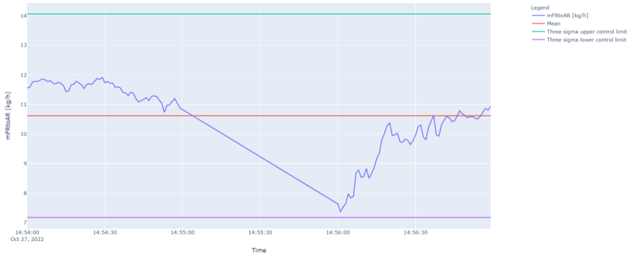
Figure 69. Timeseries graphs for fuel reactor to air reactor gas leakage at the 0.35 m bed height condition.
