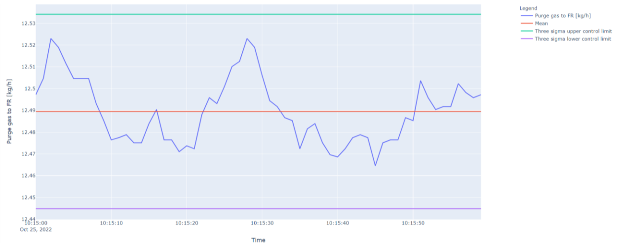
Figure 45. Timeseries graphs fate of the amount of AR/FR purge gas that moved to the fuel reactor at the base case condition (third repeat).
