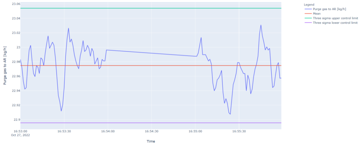
Figure 46. Timeseries graphs fate of the amount of FR/AR purge gas that moved to air reactor at the base case condition (first repeat).
