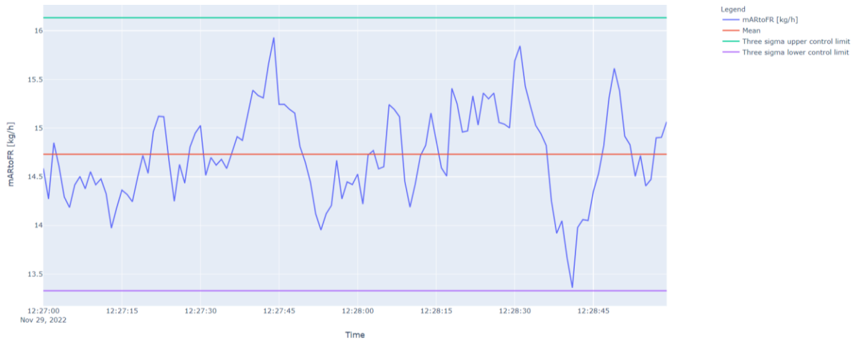
Figure 94. Timeseries graphs for air reactor to fuel reactor gas leakage at the 0.125 m weir opening height condition (second repeat).
