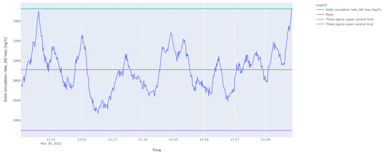
Figure 92. Timeseries graphs for solid circulation rate at the 0.125 m weir opening height condition (third repeat).
