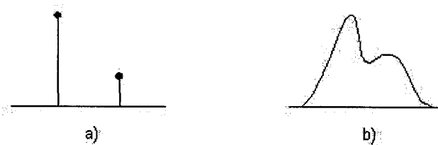
Figure 2.2: The impulse response of two path multipath channel model with specular paths (a), and the diffuse version of the channel due to scatterers (b).
