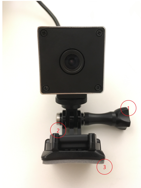
Figure 3.8: The front view of the support of the camera. (1) Long thumb screw. (2) Vertical mounting buckle. (3) Curved adhesive mount.
