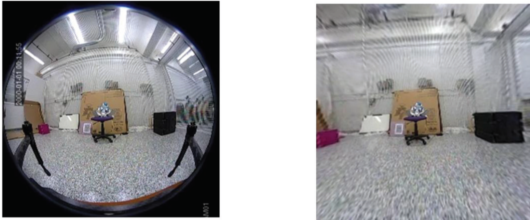
Figure 2.6: i) Original image and ii) Dewarped image [16]
