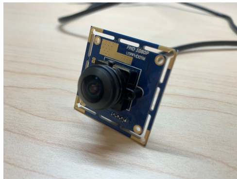
Figure 4.1: 180 degrees Fisheye Lens Wide Angle Camera
