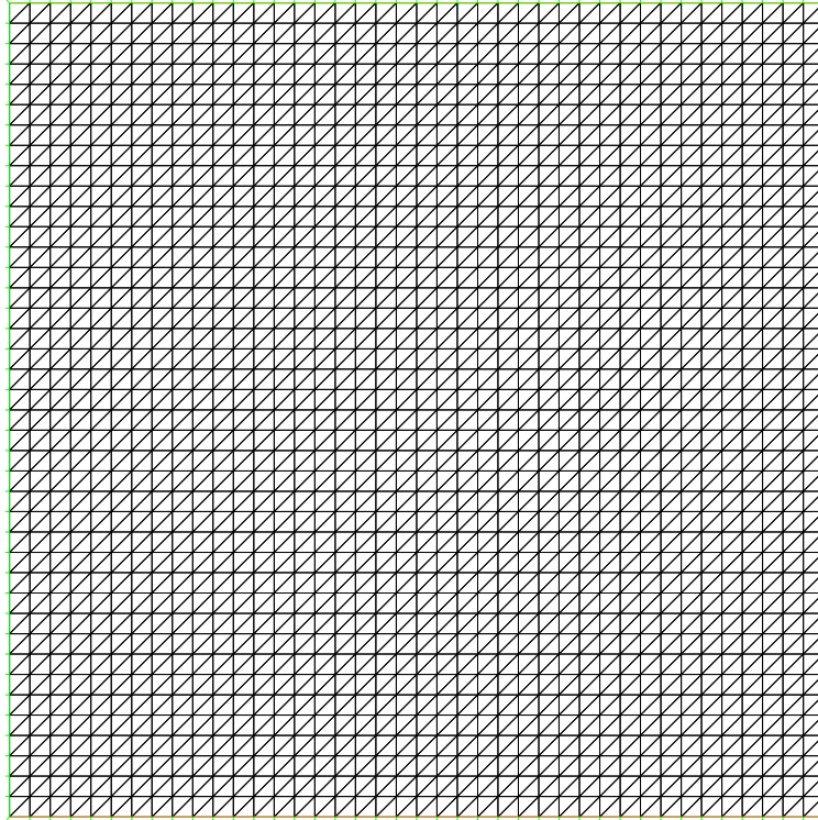
Figure 4.1: Uniform triangular mesh, 40x40 grid, 3200 elements
