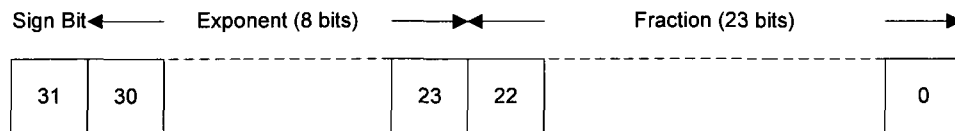
Figure 2-2 IEEE 754 Format of Floating Point Numbers
