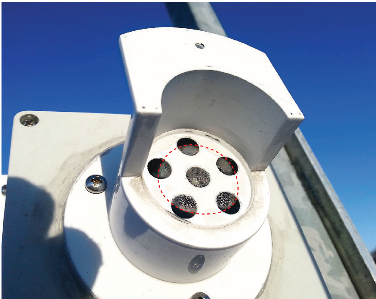
Figure 5.16: The condensation on the quartz window of the collimation tube as outlined by the dashed circle. It is one of the main factors limiting the SSIM's performance.
